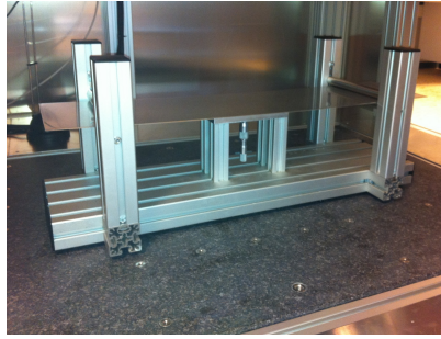
Figure 2.6: The device that was used for the testing of the setup. The micrometer screw is visible in the centre of the image.
