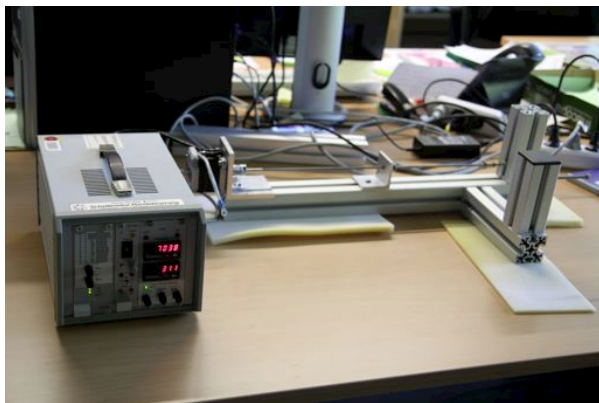
Figure 2: Coil Winding Setup.
