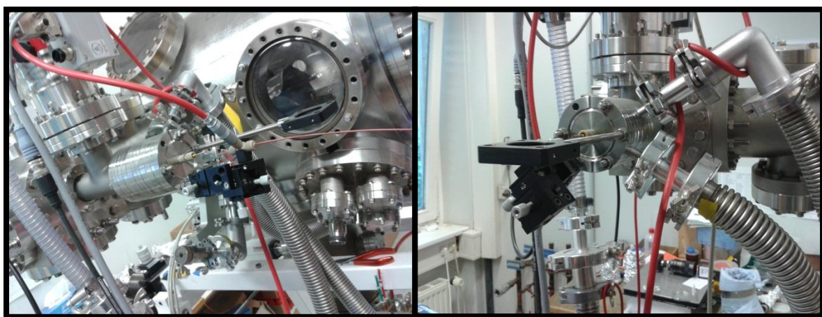
Figure 2.1: Initial conditions for the setup. In the left picture, it is possible to observe the previous unstable holder which will be replaced and the conetion between the capllary and the ESI-source (needle). In the right side of the page we can perceive the geometric restriction because of the position of the flange where our device should be fixed.
