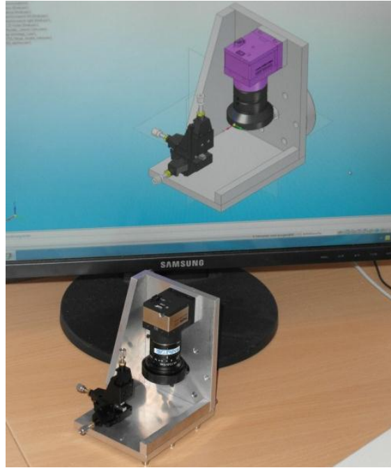
Figure 5.2: Comparison between the Solid Edge ST3 design and the real construction.
