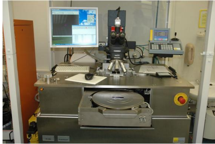
Figure 8: Karl Suss PA300 Probe Station used for module characterization.
