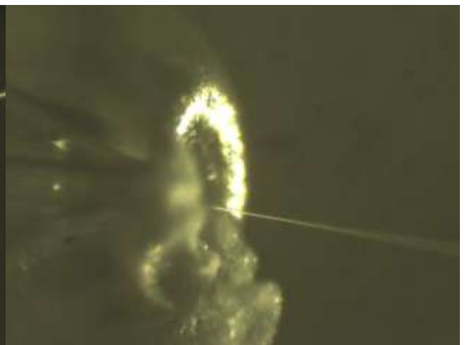
Fig. 21 NOZZLE_3 (1st configuration) jets with the sample LYSOZYME_A: 2 M NaCl, 0.1 M amm. ac., 50 g/l HEWL, pH 7, temperature 20°C, 2 μm filtered. Diameter of the jet is 5-6 microns. The gas pressure is 297 psi, the liquid pressure is 62 psi. NaCl crystal growth on the nozzle observed after 20 minutes jetting.
