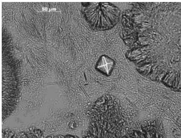
Fig. 7 Optical picture of LYSOZYME_G_F: 0.9 M NaCl, 50 g/l HEWL, 0.5 μm prefiltered, pH 8, temperature 20°C. Clear tetrahedron lysozyme crystal is observed.
