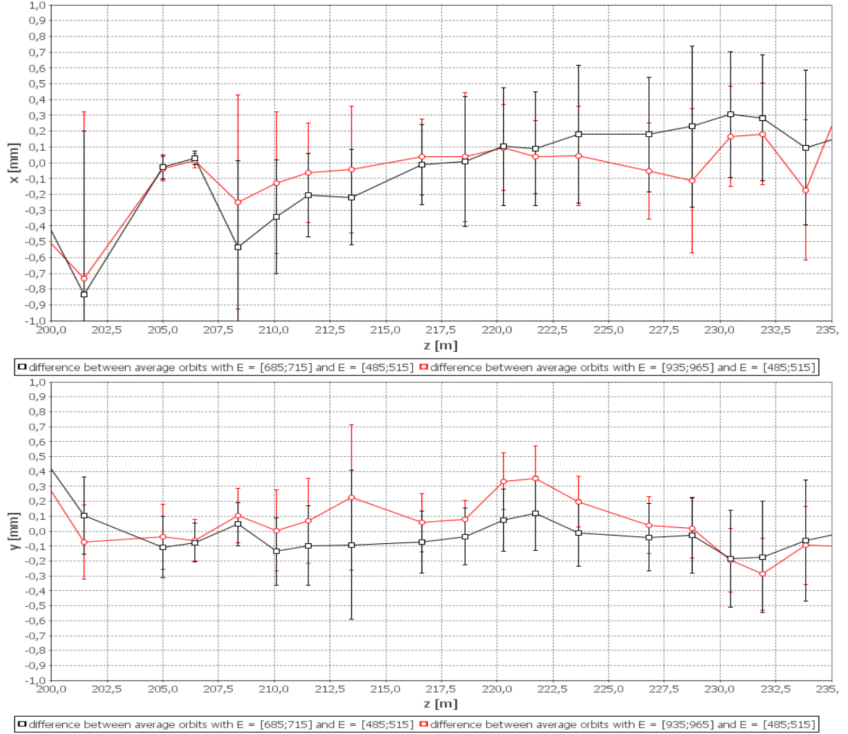
Figure 4. The difference between average orbits with E = [685;715] MeV; E = [935;965] MeV and average orbit with E = [485;515] MeV
