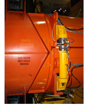
Figure 6: Left: Ratio of the average channel response measured with and without magnetic field of all channels in CASTOR. Channels shown in gray have no signals because of the magnetic field influence (mod - 7 - 10) or due to a hardware failure. Right: Assembly gap (arrow-like) between the rotating and collar shielding of CASTOR.
