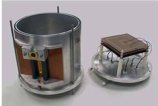
Figure 11: Experimental setup of the 'Small TPC' operated with a double GEM stack (on the right).
