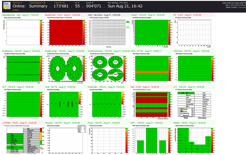
Figure 1: DQM GUI - Data Quality Monitoring Graphical User Interface - This webserver is used to store the histograms which are obtained from data harvesting and are used to check the validity of the data. These histograms are available to anyone with CMS credentials.
