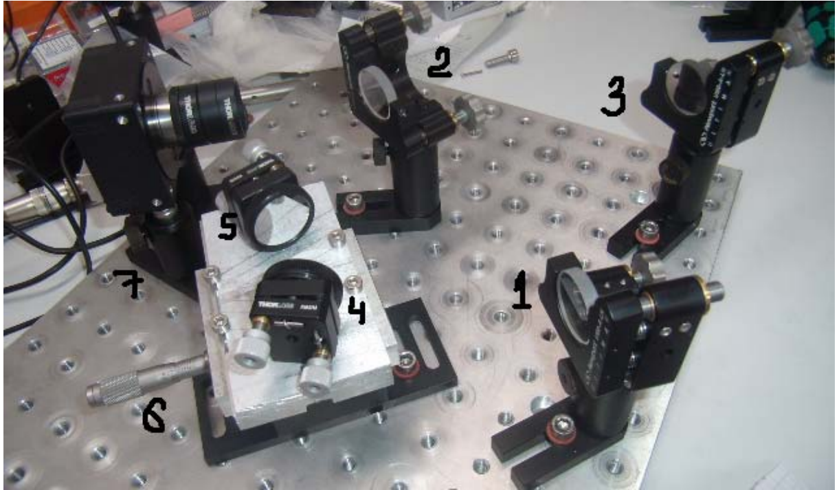
Figure 9. Experimental setup. Modified Mach-Zehnder type interferometer
