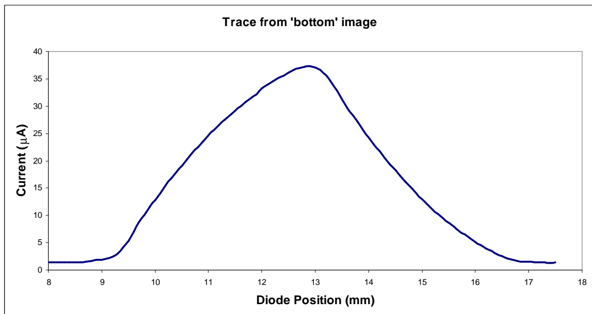
Figure 2.3d – Trace from region of unreflected image. The bottom edge of the image is at 9.3mm, giving \Delta s = 66.4\text{mm} , which is about 3mm smaller than expected for an angle of 5^\circ . The top of the image is much harder to find, as it is not the peak (due to the circular nature of the beam, the current is decreasing before the peak is reached), and the right edge of the trace goes to zero fairly slowly.
