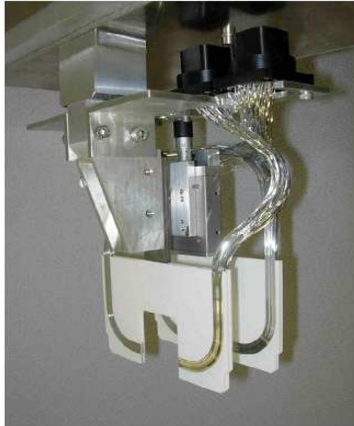
Figure 6: ALFA Overlap Detector. There are 30 fibers on each side of the plate.
