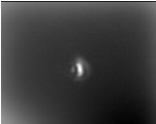
Figure 5: real picture obtained with the CCD camera at z = 25\text{mm} ( \lambda = 52\text{ }\mu\text{m} ).
