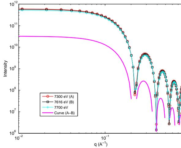
Figure 7: Scattering intensity patterns for 'onion' nanoparticle at energies below and near the K absorption edge of Co and subtraction curve of two scattering patterns at two energies in loglog scale.
