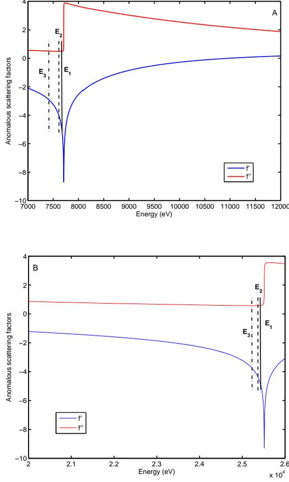
Figure 2: Anomalous scattering factor for (A) Co and (B) Ag absorption edge.
