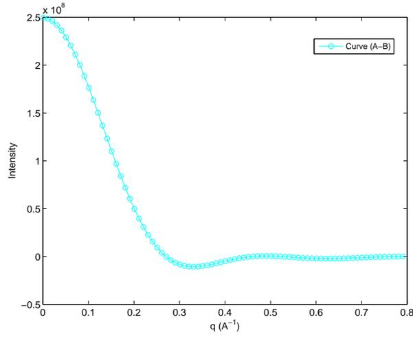
Figure 5: Subtraction curve in linear scale of two scattering intensity patterns at two energies at cobalt edge.
