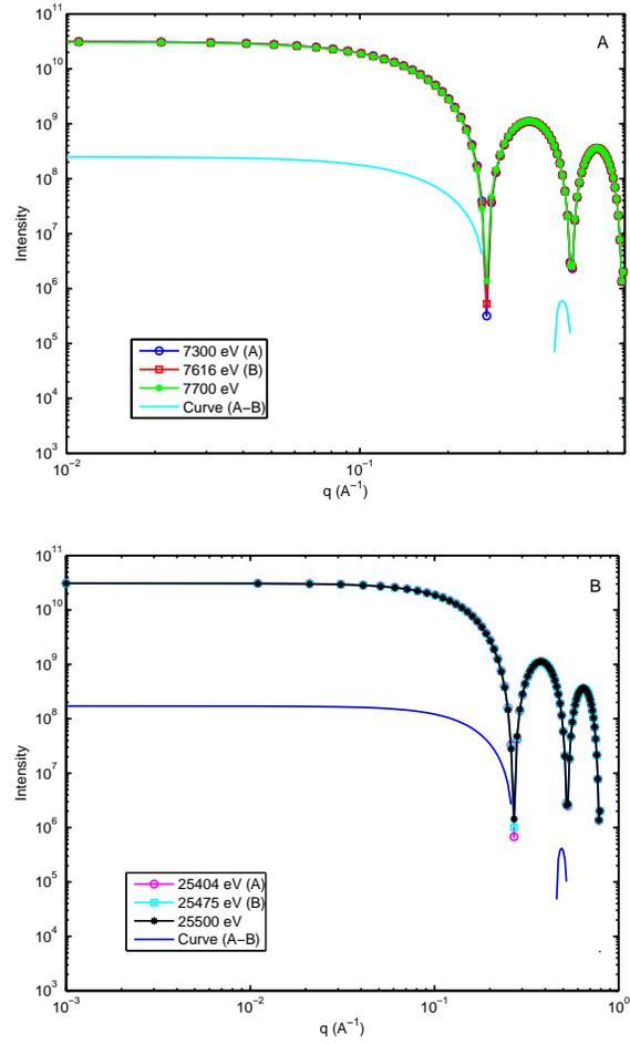
Figure 4: Scattering intensity patterns for core-shell nanoparticle at energies below and near the K absorption edge of Co (A) and Ag (B) elements and subtraction curve of two scattering intensity patterns in loglog scale.
