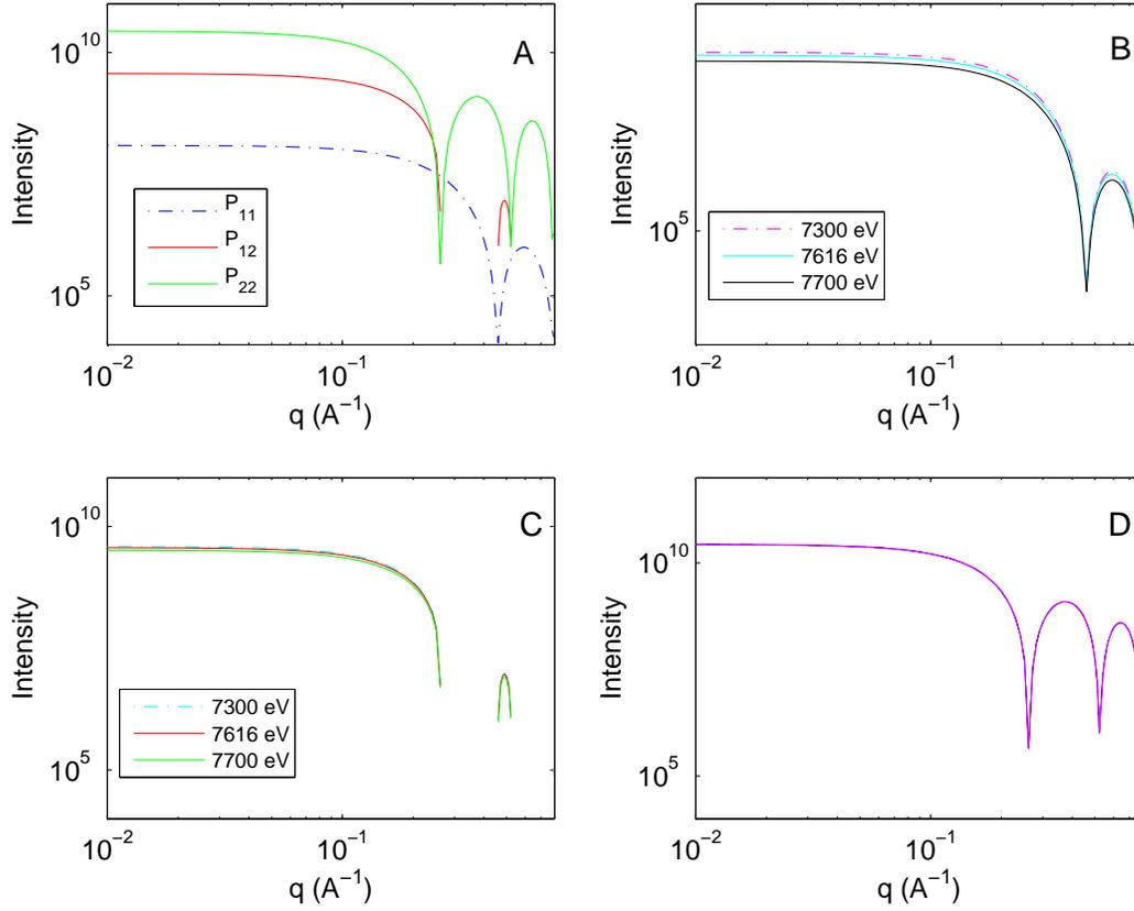
Figure 3: (A) Partial structure factors of Co-Ag core-shell at 7616 eV for Co energy; (B), (C) and (D) shows, respectively, the  $P_{11}$ ,  $P_{12}$  and  $P_{22}$  term for three energies below and near the cobalt absorption edge. Note that in the last graphic there was a superposition of the curves at different energies.
