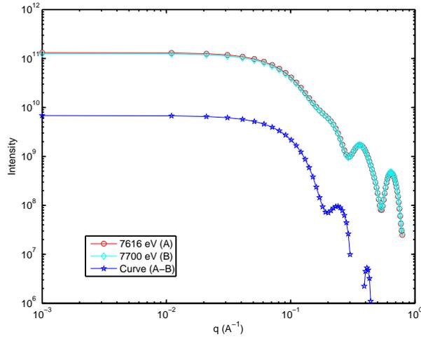
Figure 10: Scattering patterns and subtraction curve coming from polydisperse system at cobalt absorption edge.
