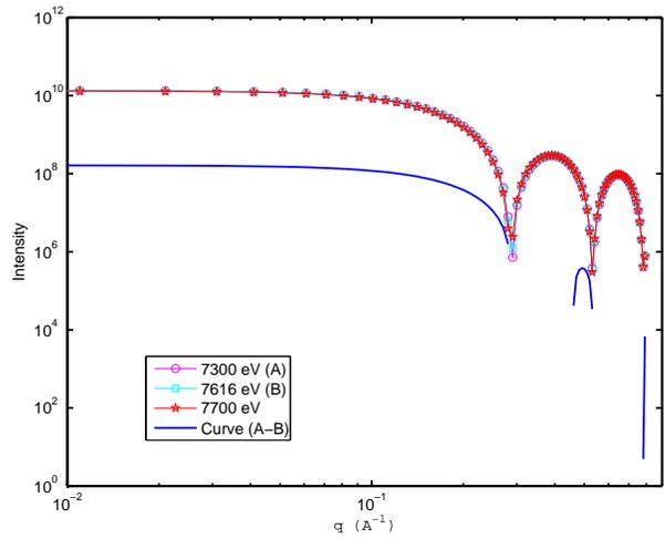
Figure 6: Scattering intensity patterns for core-shell nanoparticle with core and shell constituted by cobalt and silver, respectively at Co absorption edge.
