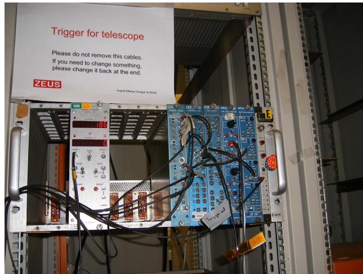
Figure 6: The telescope trigger coincidence logic and gate generator
