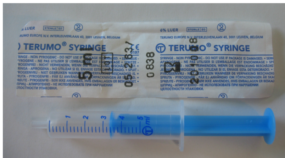
5 ml Syringe, Diameter 12.2mm, max Infusion Rate: 22.289ml/min
