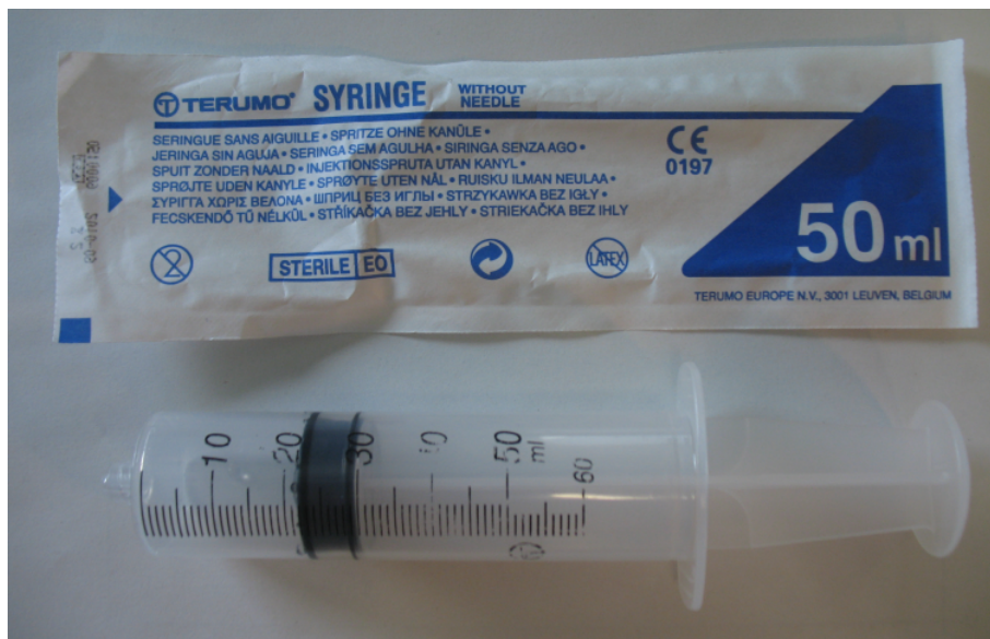
50 ml Syringe, Diameter 29.5mm, max Infusion Rate: 130.32ml/min
