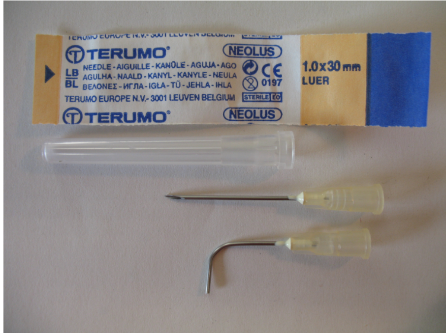
Hypodermic needle, before and after preparation. Needle aperture: 1 mm
