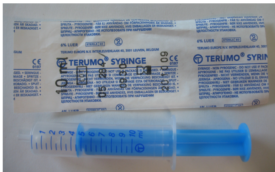
10 ml Syringe, Diameter 16.2mm, max Infusion Rate: 39.302ml/min
