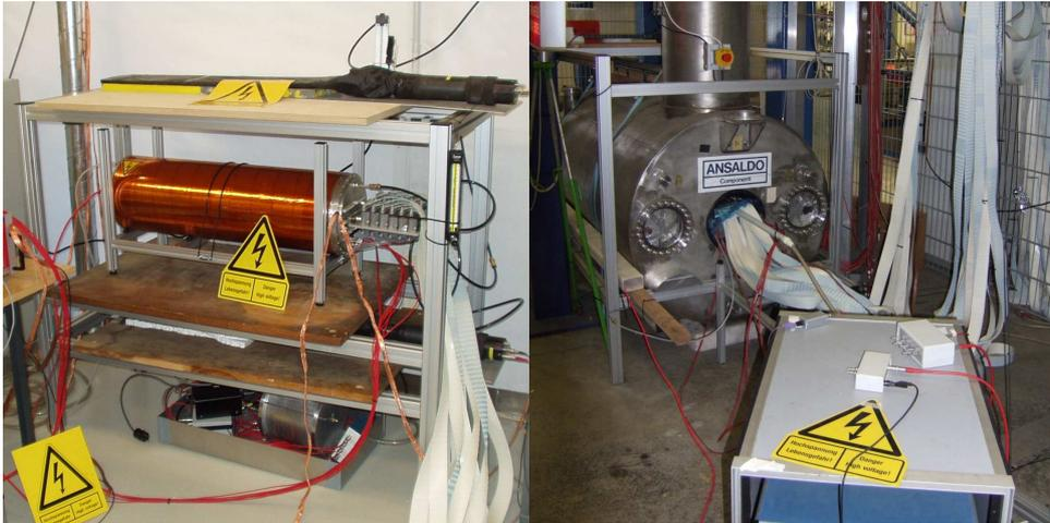
Figure 3: Photo of the MediTPC prototype (left) and the MediTPC inside the magnet (right)
