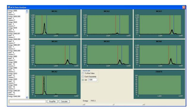
For spectra from each channel, markers can be set to integrate only through data from selected scope. There is provided additional window only for setting markers.
