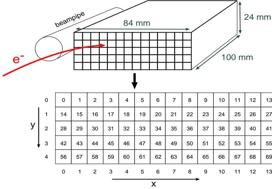
Figure 2: *The 6 meter tagger*
