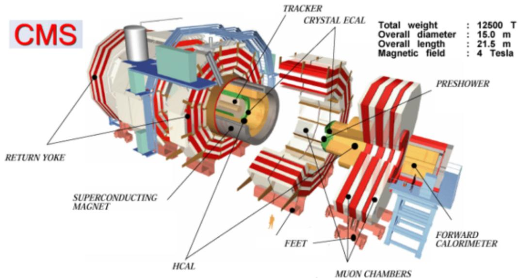
Figure 1: 3D drawing of CMS detector [1]
