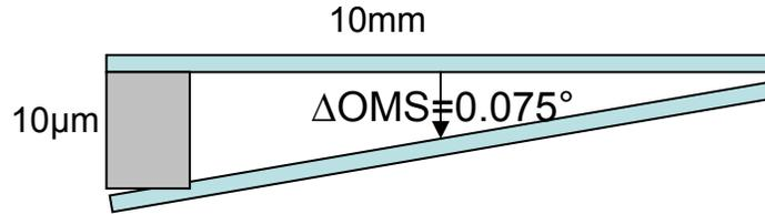
**Figure 7:** *The two wafers are not exactly parallel*
