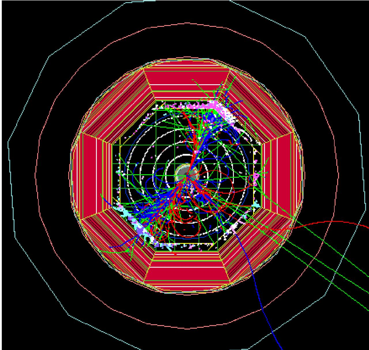
**Geant4 simulation of Higgs event in SiD detector, using MOKKA framework including geometry DB for SiD concept**
