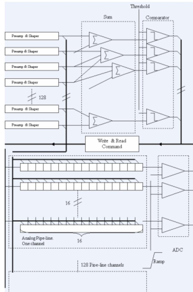
Next step: going to 128 channels with analogue sampling included; second chip prototype currently under design, foreseen submission Fall 05. Will equip the test beam prototypes
