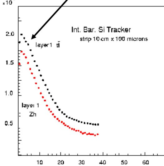
**Occupancies are calculated with BRAHMS full simulation (Si-Envelope+TPC), Higgstrahlung HZ with bbbar and q qbar at Ecm=500 GeV
