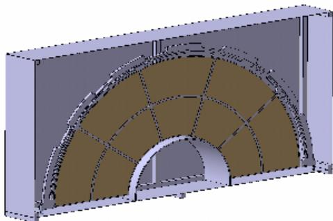
preliminary design of the mechanical prototype to test the cooling system for a disk of the inner forward
