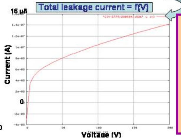
**Test of 10 Hamamatsu det. S8743 (GLAST)
