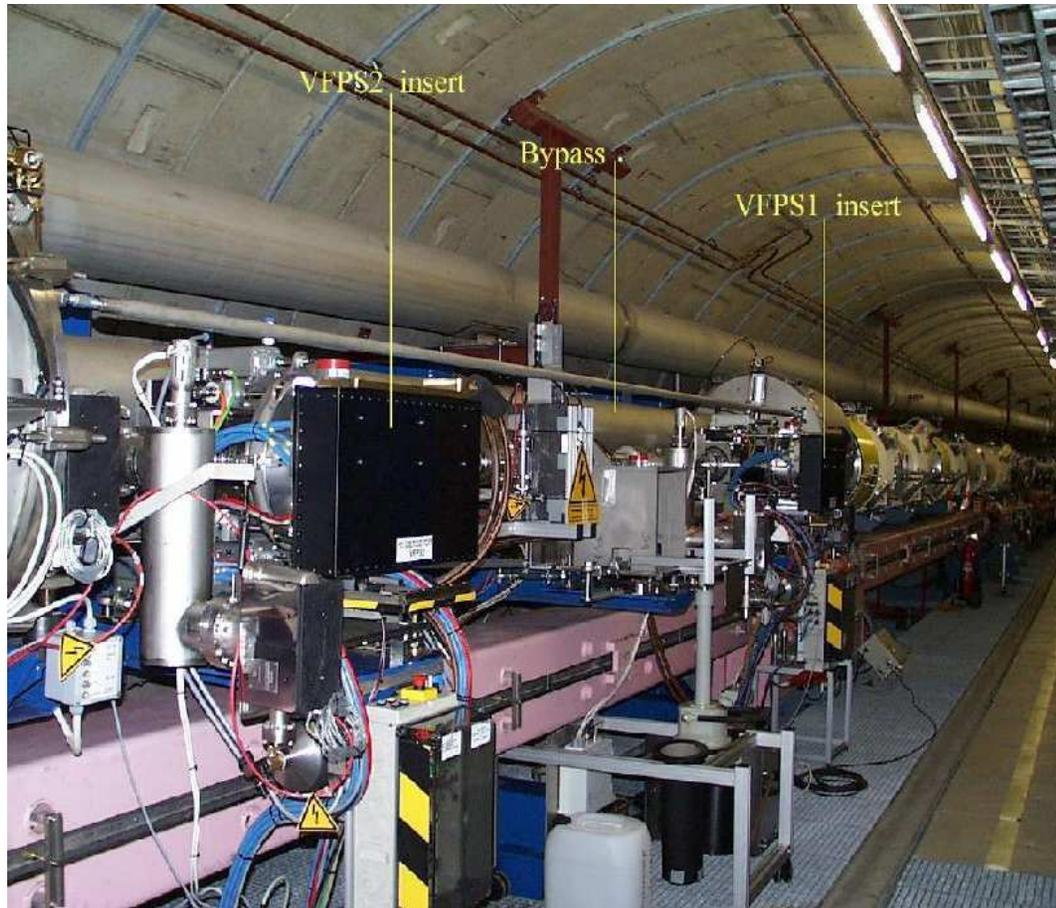
Very Forward Proton Spectrometer installed in HERA tunnel (at 220 m).
