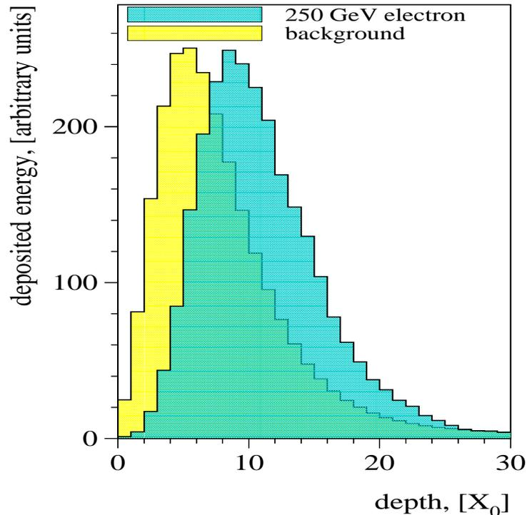
Figure 15: The shapes of the longitudinal energy distributions of electrons from beamstrahlung (background) and a single electron of 250 GeV.
