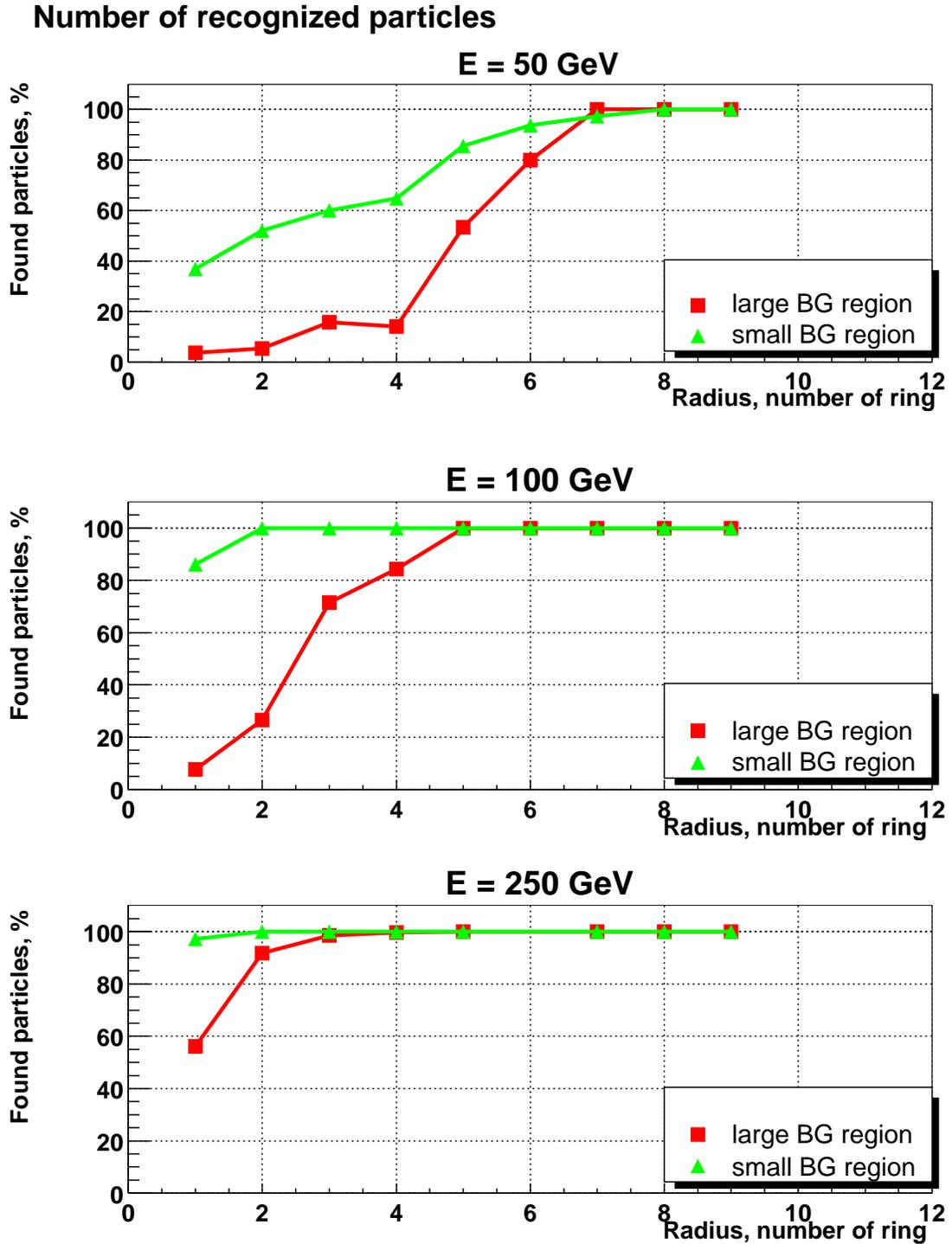
Figure 24: The efficiency to identify an electron of energy 50, 100 and 250 GeV as function of the radius in the large background region (squares) and the low background region (triangles).
