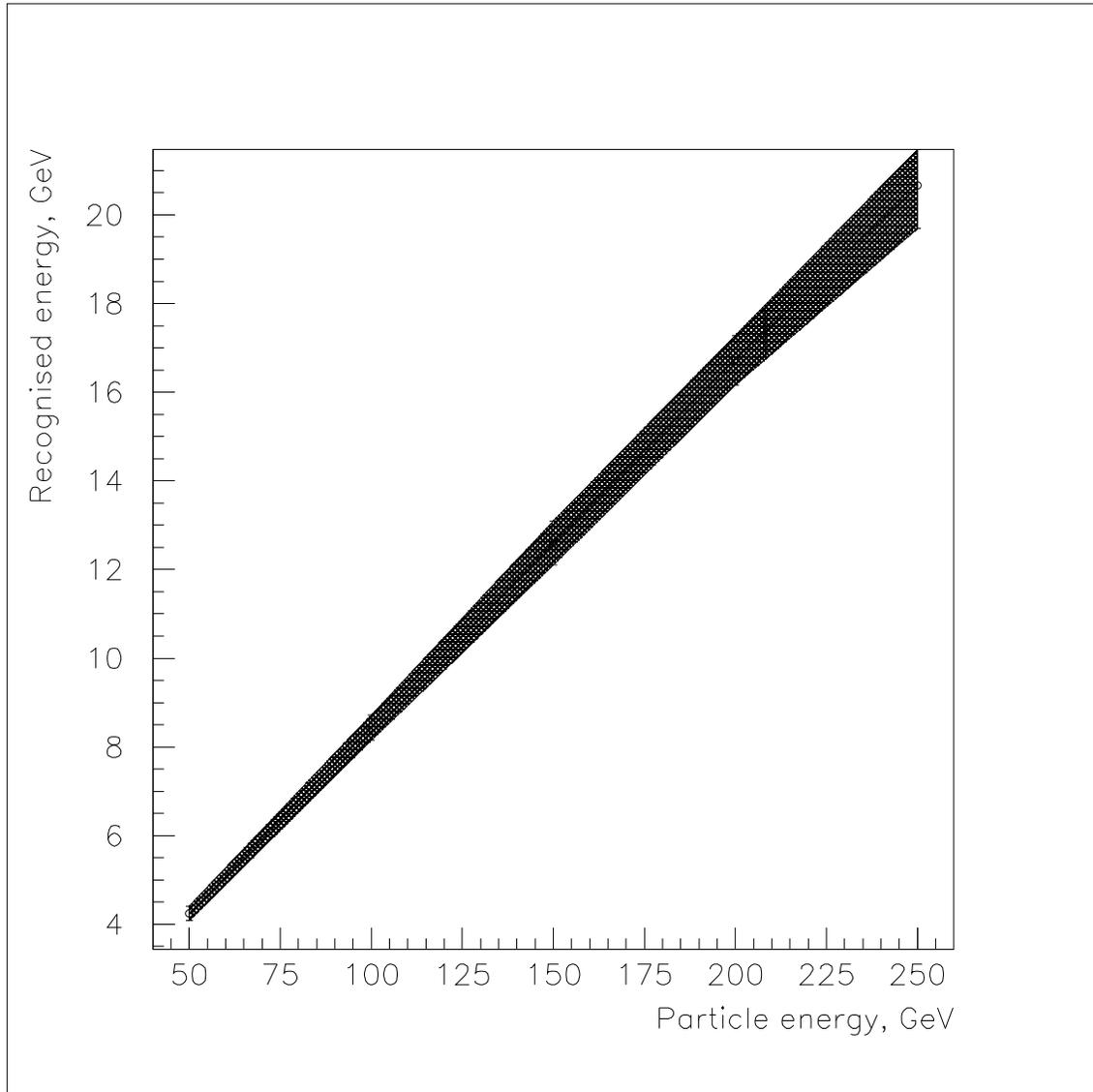
Figure 25: The energy measured in the calorimeter as function of the initial electron energy.
