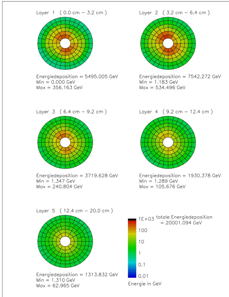
Figure 29: The energy depositions of electrons from beamstrahlung (background) in the crystal calorimeter for several segments in depth.
