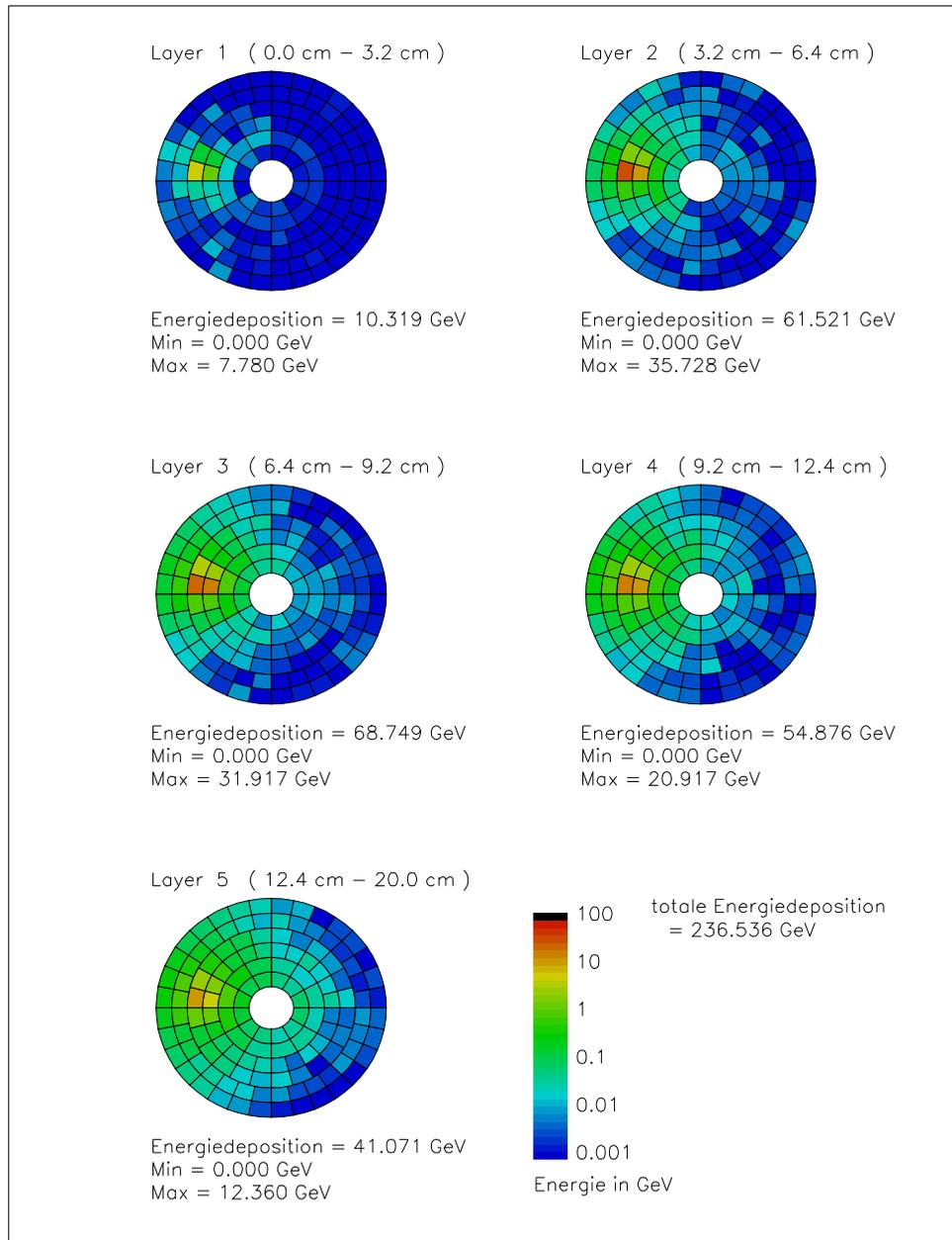
Figure 28: The energy depositions of a shower induced by a 250 GeV electron in the crystal calorimeter for several segments in depth.
