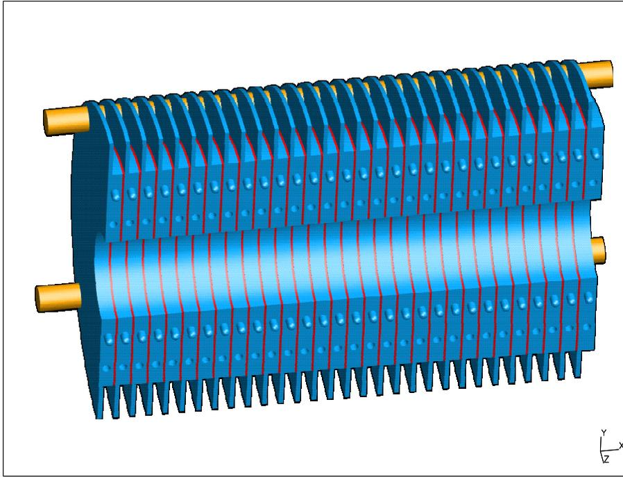
Figure 16: The structure of a half barrel of the sandwich calorimeter. Among the tungsten disks diamond sensors are interspersed.
