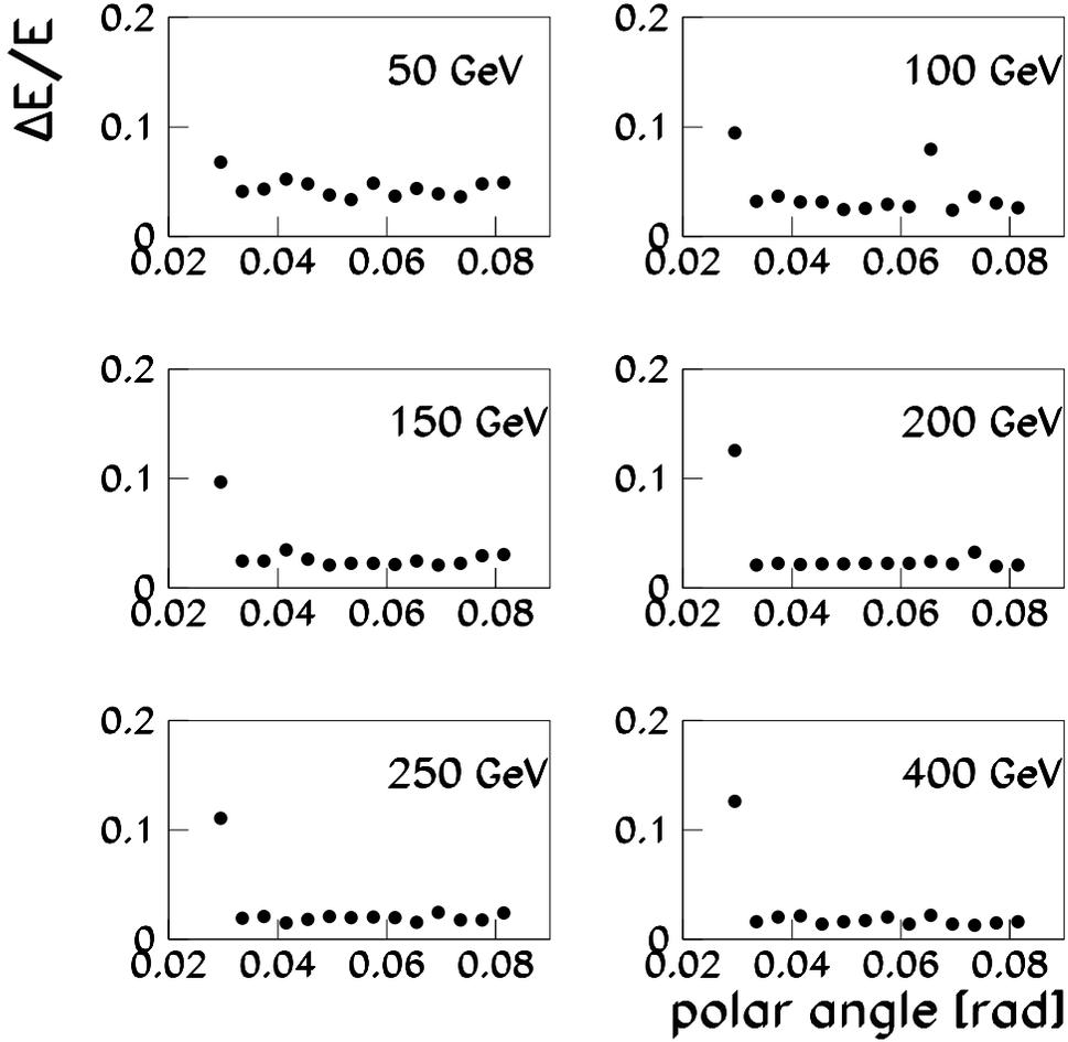
Figure 12: The energy resolution of LAT as functions of  $\theta$  for several particle energies.
