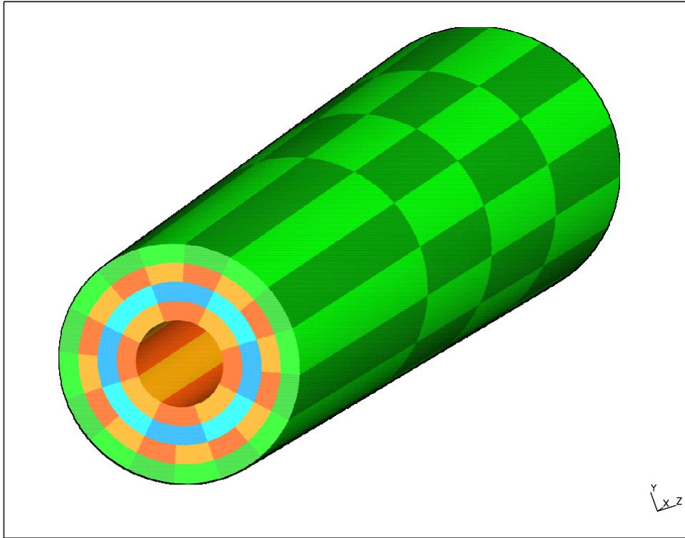
Figure 20: The structure of the crystal calorimeter. The rings consist of segments which are longitudinally subdivided into pieces.
