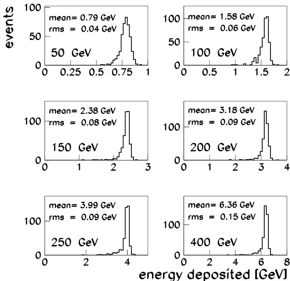
Figure 7: The total energy deposited in the silicon sensors of LAT.
