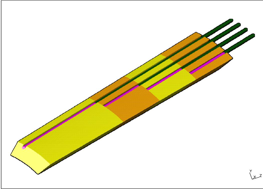
Figure 21: Scintillator pieces forming a segment of the crystal calorimeter. Each piece is connected to an optical fibre, which crosses, optically isolated, the crystals to the rear side of the calorimeter.
