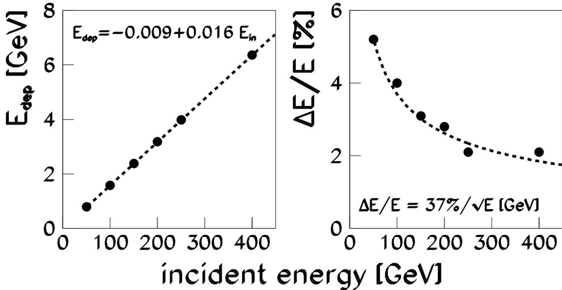
Figure 8: The energy response(left) and the energy resolution(right) of LAT as functions of the particle energy.
