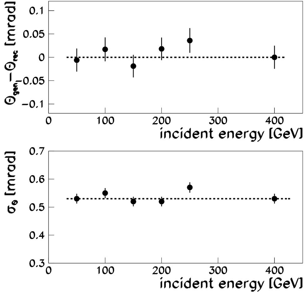
Figure 13: The reconstruction of  $\theta$ . The difference of the generated and reconstructed angles (left) and the standard deviation of the reconstructed angle (right) as functions of the particle energy.
