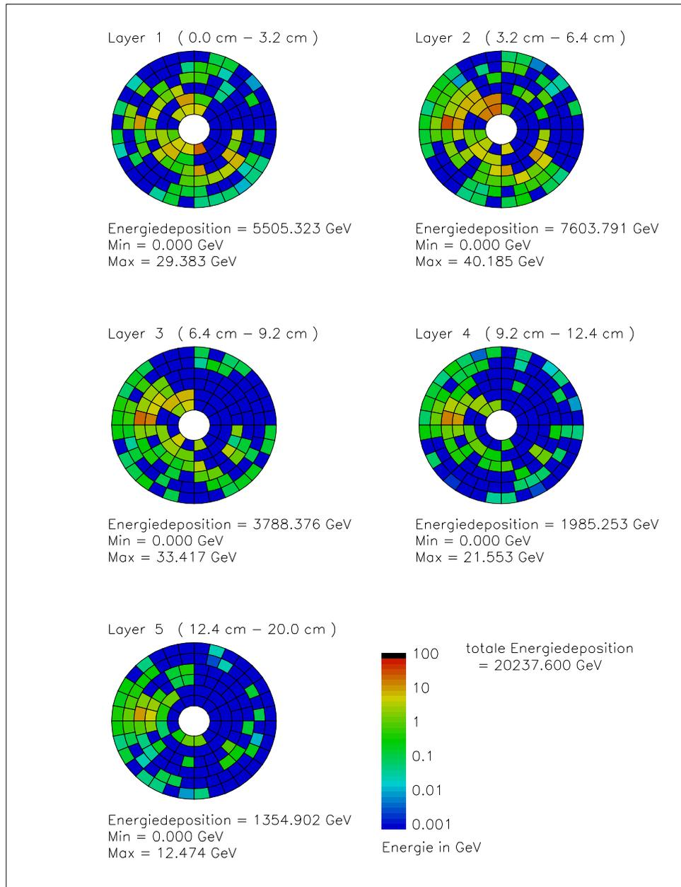
Figure 31: The difference between the depositions from an electron of 250 GeV superimposed on the background and the background obtained from the calorimeter on the opposite side.
