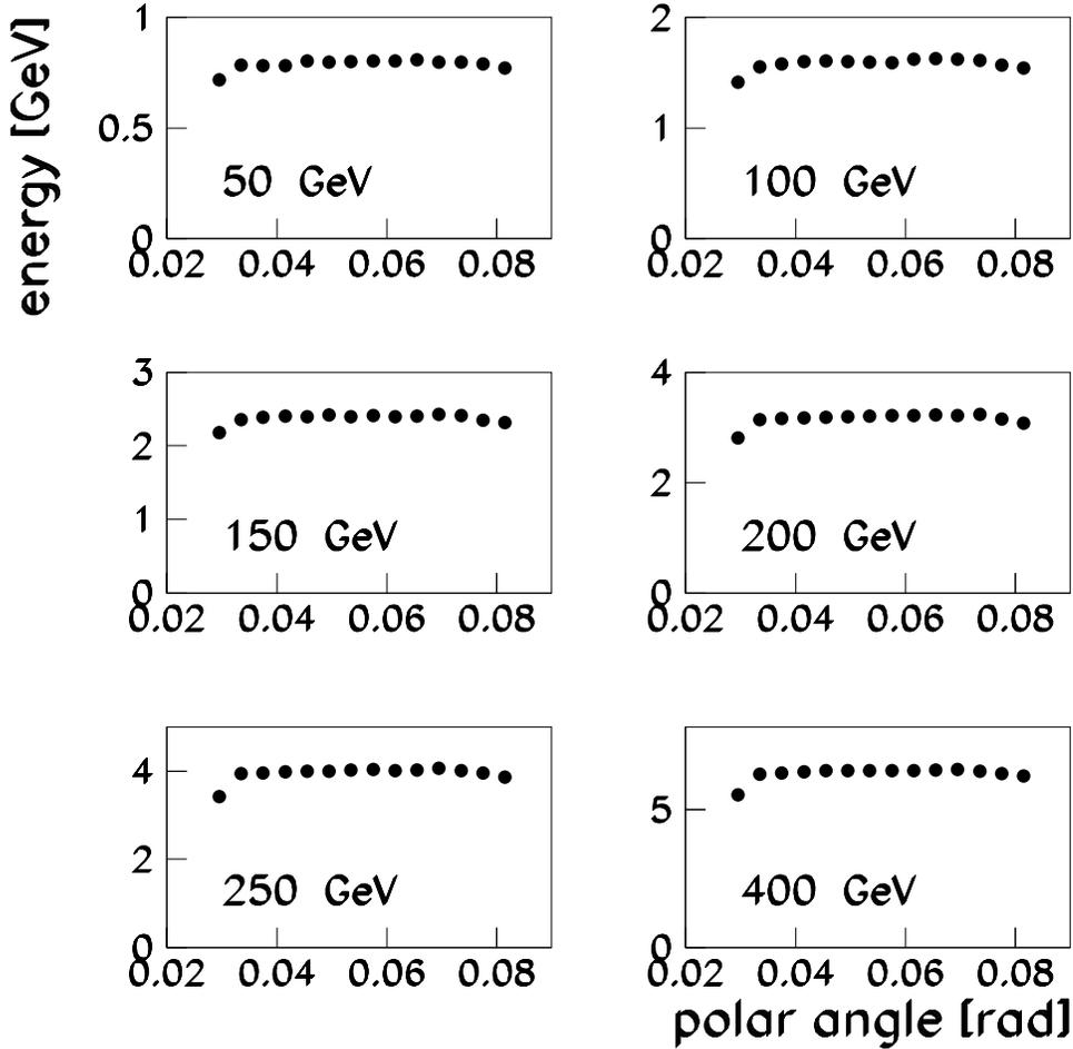
Figure 11: The energy response of LAT as functions of  $\theta$  for several particle energies.
