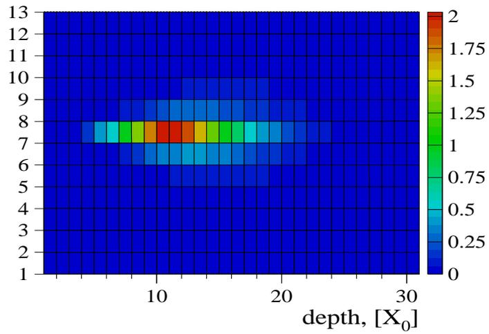
Figure 23: The transversal (top) and longitudinal (bottom) projections of the shower of a 250 GeV electron in the sandwich calorimeter. The scale on the right side is in GeV.
