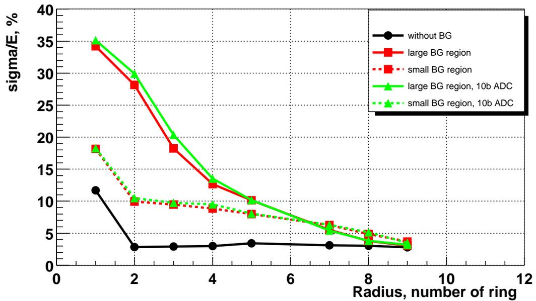
Figure 26: The resolution of the energy measurement in the calorimeter for electron energies of 100 and 250 GeV as function of the radius. Black dots correspond to the case of no background, the dashed lines to the small background and the solid lines to the large background regions. Squares are obtained before and triangles after digitisation using an ADC with 10 bit resolution.
