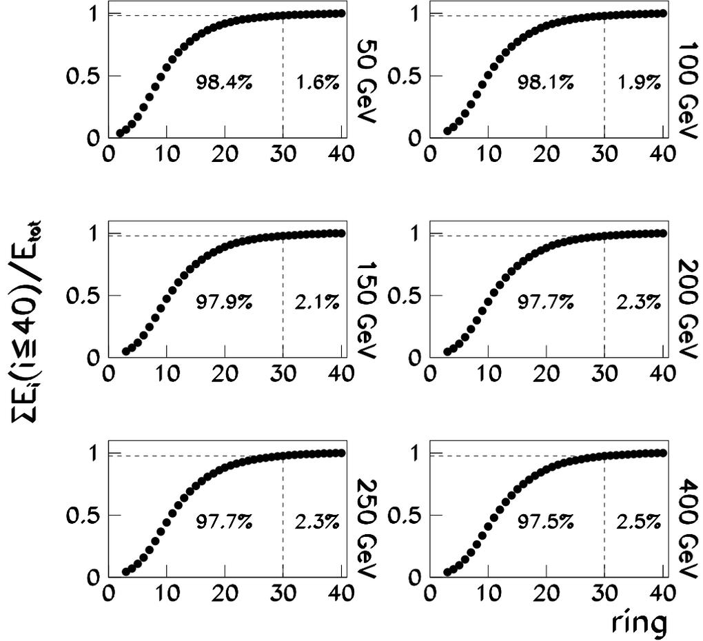
Figure 10: The cumulated energy fraction deposited versus number of layers (“rings”).
