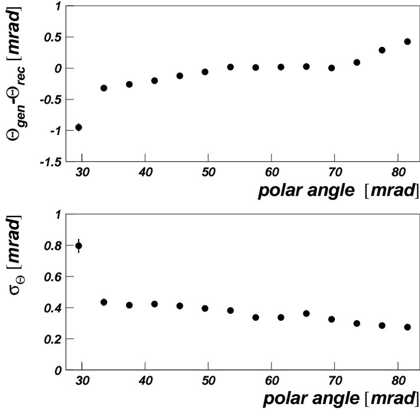
Figure 14: The reconstruction of  $\theta$ . The difference of the generated and reconstructed angles (left) and the standard deviation of the reconstructed angle (right) as functions the  $\theta$  angle.
