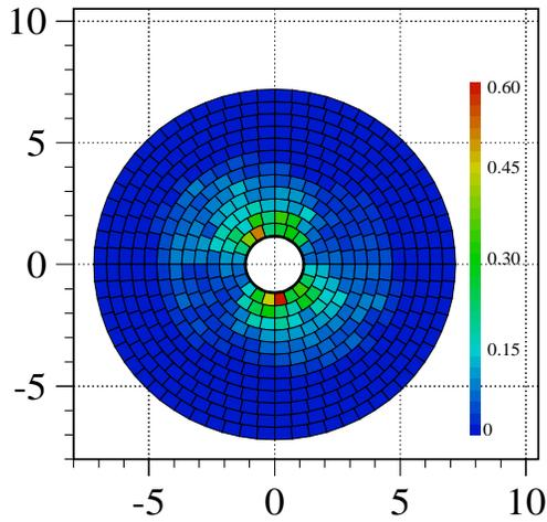
Figure 22: The average background per pad in one layer of the sandwich calorimeter (top) and the standard deviation obtained from 10 bunch crossings (bottom). The scale on the right side is in GeV.
