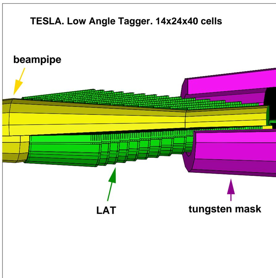
Figure 6: The LAT calorimeter (green). The cut shows its structure. The LAT is mounted just outside the beam pipe (yellow). The tungsten mask (red) and the graphite absorber (black) are also visible.
