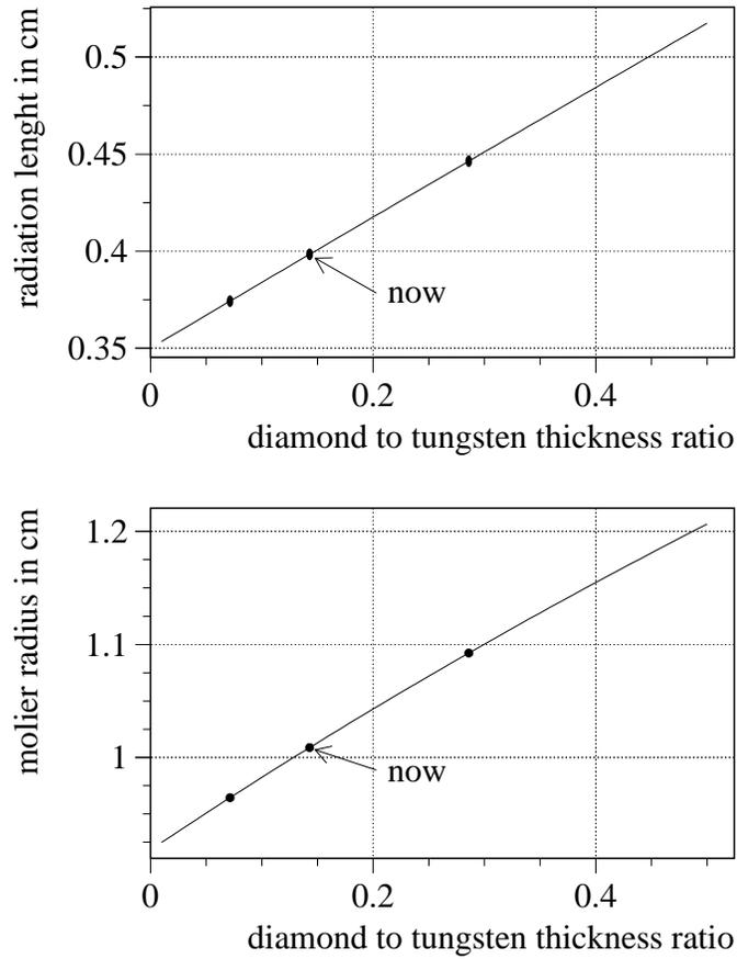
Figure 17: The dependence of the radiation length and the Molière radius on the ratio of sensor and absorber thickness. The arrow points to the current design. The dots left and right indicate the values of the radiation length and Molière radius after changing the thickness ratio by a factor of two.
