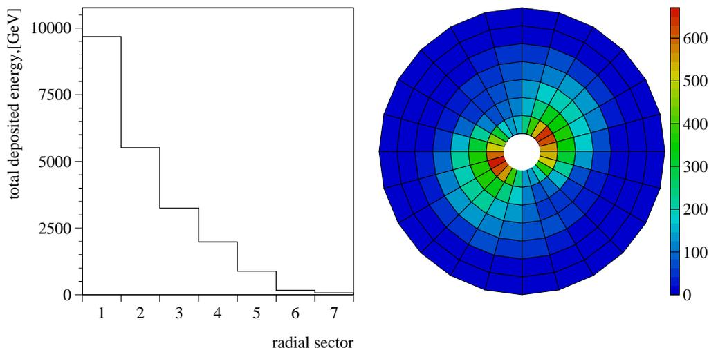
Figure 5: The energy deposition in the LCAL induced by beam background as function of the distance from the beam pipe (left) and in the plane perpendicular to the beam (right). The centre-of-mass energy is 500 GeV and standard machine parameter are used [1]. Each radial sector corresponds to about 1 cm. The units on the right scale are GeV.
