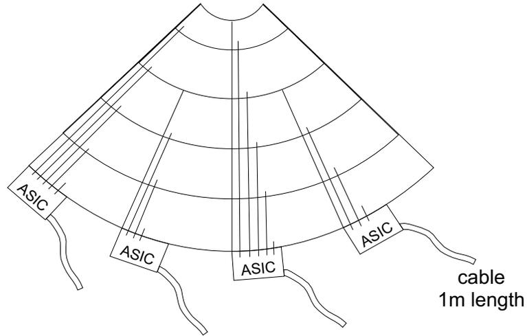
Figure 19: The readout of the sensor pads using a capton printed circuit connected to ASIC preamplifier.
