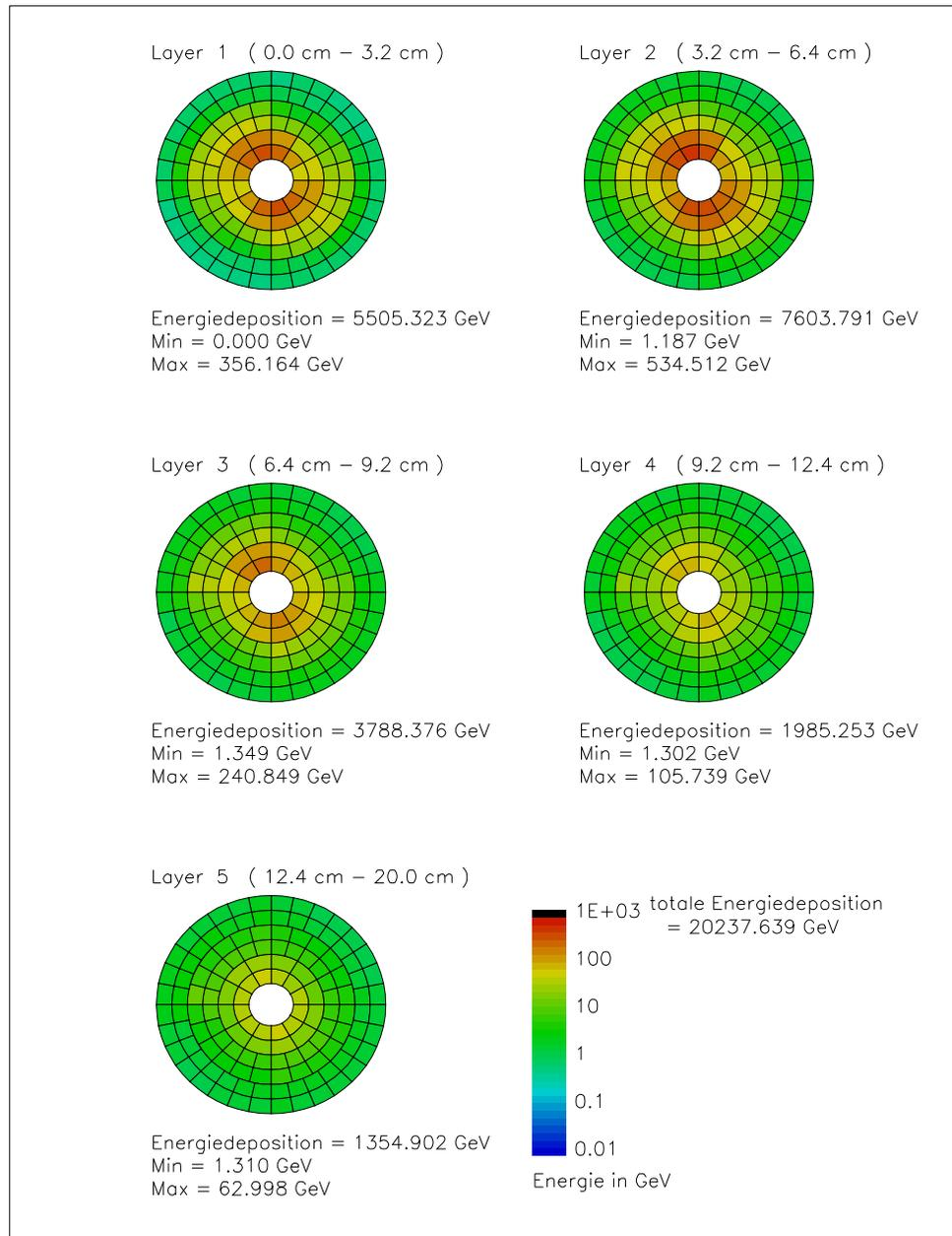
Figure 30: The superposition of the shower of an electron of 250 GeV and the electrons from beamstrahlung in the crystal calorimeter for several segments in depth.
