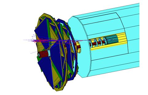
Simulated primary electron which has started an electromagnetic shower in the endplate of the Central Tracking Detector (CTD). Also shown is the barrel and forward part of the MVD.
