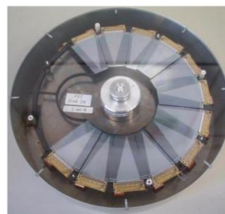
The new **Forward Silicon Tracker (FST)** consists of 12 single-sided silicon planes measuring tracks in 3 projections in the range from  $7^\circ$  to  $17^\circ$ . A radial plane shown here has 640 strips between 6 and 12 cm radius. The elliptical and excentric beam pipe accommodates only 12 of 16 azimuthal sectors.
