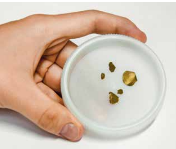
Two-dimensional layered crystals of tantalum disulphide grown at Kiel University. This quantum material has a flaky structure similar to that of graphite.
