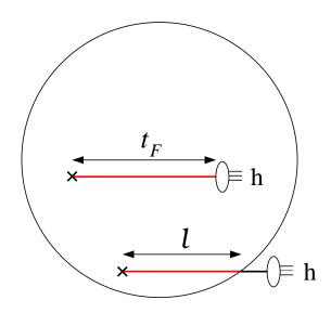
$$L = t_f \times \left[1 - \frac{3}{8} \frac{t_f}{R} + \frac{1}{64} \left(\frac{t_f}{R}\right)^3\right] \qquad t_f \le 2R$$
