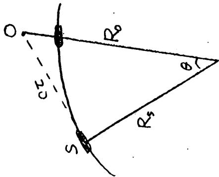
$$F_{\theta 0} = -e \left( \frac{1}{R_0} \frac{\partial \Phi}{\partial \theta} + \frac{1}{c} \frac{\partial A}{\partial t} \right)$$
