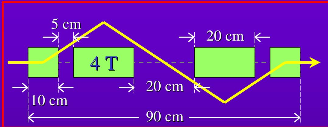
Add Super-Conducting wiggler prior to BC2 to increase incoherent energy spread ( $\times 10$ )
