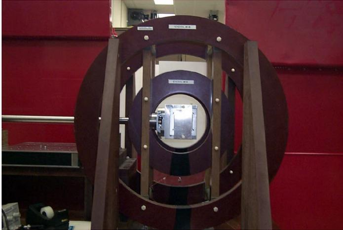
Helmholtz Coil – magnet block measurement
