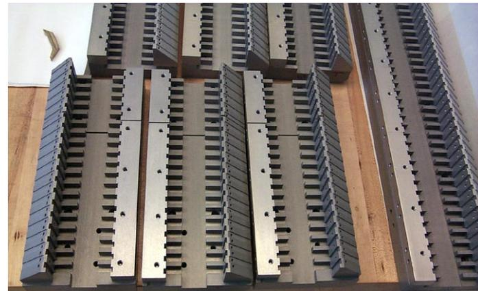
Magnet block clamping fixtures
