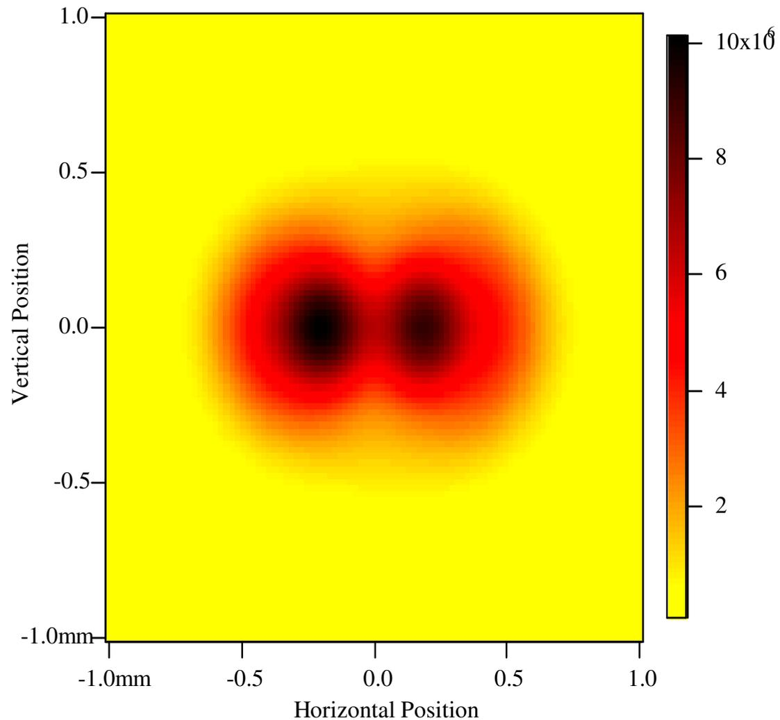
Calculated spatial distribution of the undulator radiation from a three-undulator cell with a missteering  $q_{mis} = 4 \mu\text{rad}$ , an electron beam emittance of  $0.05 \text{ nm}\cdot\text{rad}$ , and a photon energy of  $8.29 \text{ keV}$ , at  $60 \text{ m}$  from the undulators.
