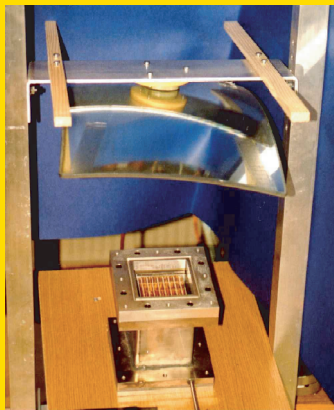
The chamber was illuminated indirectly by shining the UV lamp onto the spherical mirror
