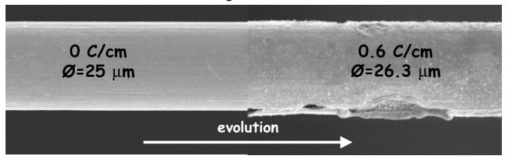
e-microscopy  $\Rightarrow$  gain loss was due to wire swelling
