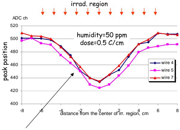
Inspite of the homogeneous irradiation intensity profile, the gas gain loss increases towards the center of the irradiated region
