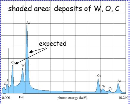
W deposited on cathode was probably etched away in irradiation area
