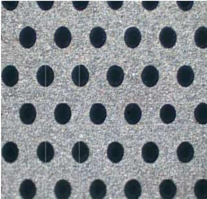
Irradiated area of the GEM after aging test
