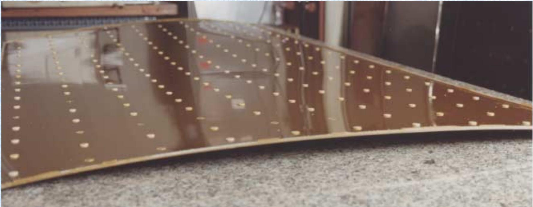
It is clearly evident from the picture the mechanical stress of the gap as well as the grid of spacers
