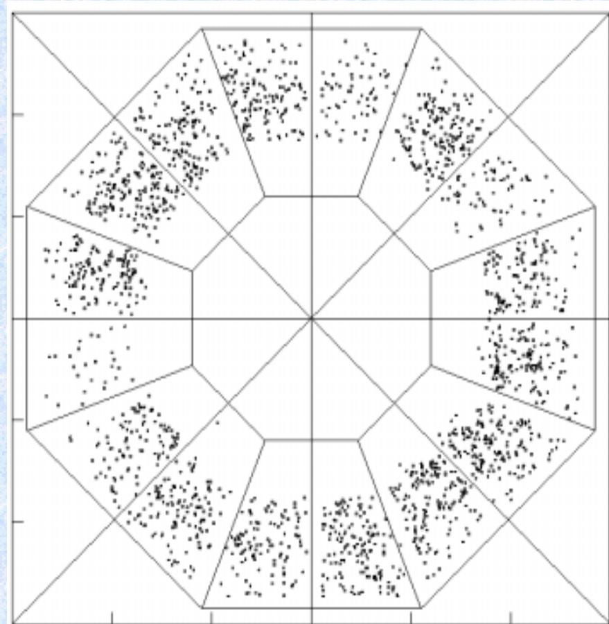
Example of muon tracks impact point on the FO plane of the spectrometer
