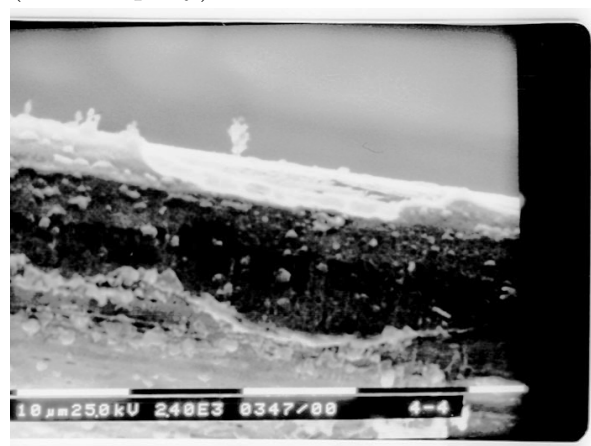
Figure 13: Deposits on anode wire (DME+epoxy).
