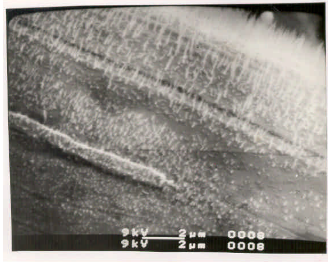
Figure 7: Deposits on anode wire at very small dose of irradiation.
