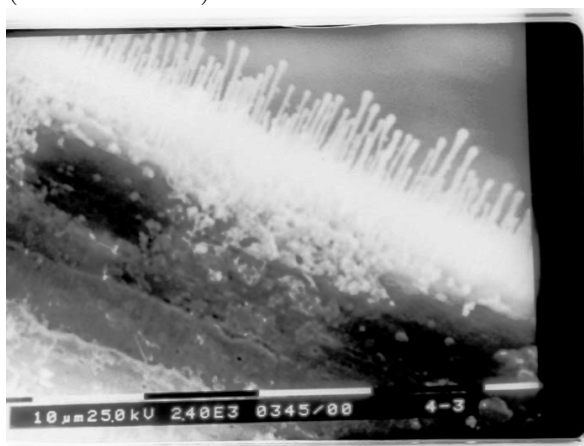
Figure 12: Deposits on anode wire (DME+Teflon).
