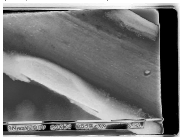
Figure 15: Deposits on anode wire ( \text{CO}_2 /Isobutane + PVC).
