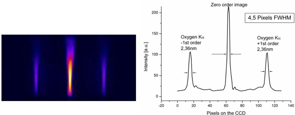
Fig. 1 CCD Image (left) and lineout (right) of zero and 1<sup>st</sup> order of O-K $\alpha$  radiation as a resolution test.
