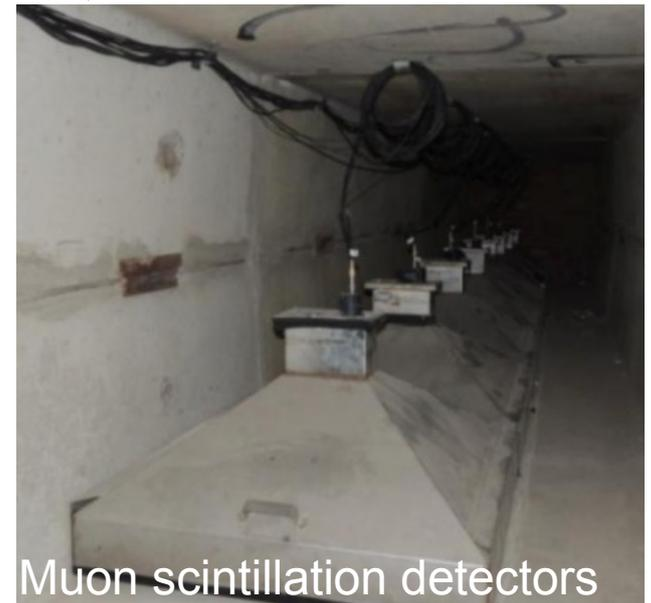
Muon scintillation detectors
