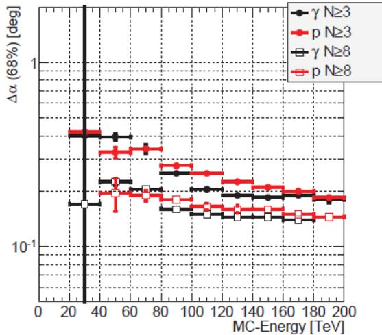
Angular resolution VS triggered stations
