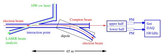
Asymmetry depends on vertical position  $\eta = \eta(y)$ ,  $y = r \sin(\phi)$ Flip laser helicity  $(-S_3)$  and  $(+S_3)$  to control systematic uncertainties Beam polarisation: proportional to mean asymmetry  $\langle \eta \rangle$  at intermediate energies
