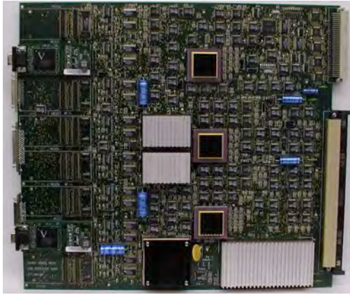
Figure 1: Front of a Receiver Card showing two Receiver Mezzanine Cards in place and Adder ASICs.
