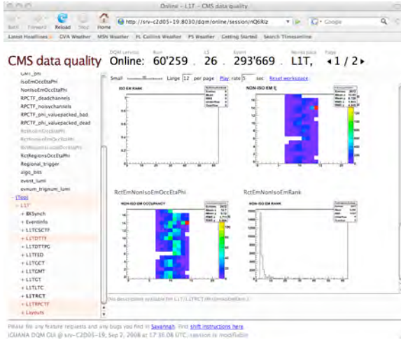
Figure 9: Online DQM browser window for a recent run. Calorimeter triggering was with the ECAL barrel. Two ECAL modules were out for the run and can be seen as white space in the two occupancy plots. Each RCT region is a single square.
