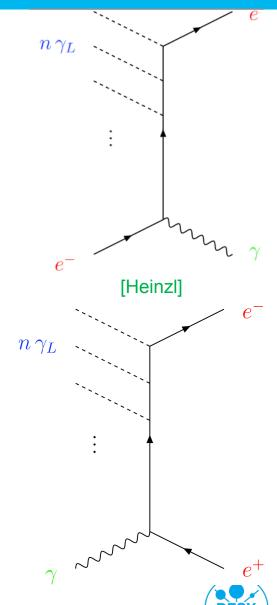
SLAC E144 studied non-linear Compton and stimulated pair production in the collision of a 46.6 GeV electron beam (the Final Focus Test Beam) with terawatt photon pulses of 1053 nm and 527 nm
