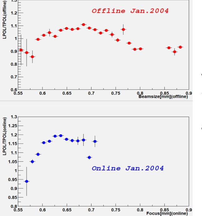
With eta-y free, the new offline method can not absorb beam size dependence yet.
