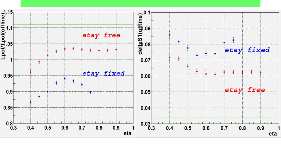
The new offline method is unstable with eta-y parameters fixed.
