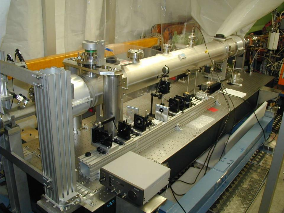
Synchrotron isolation : 3 mm of lead Thermic isolation with aluminium
