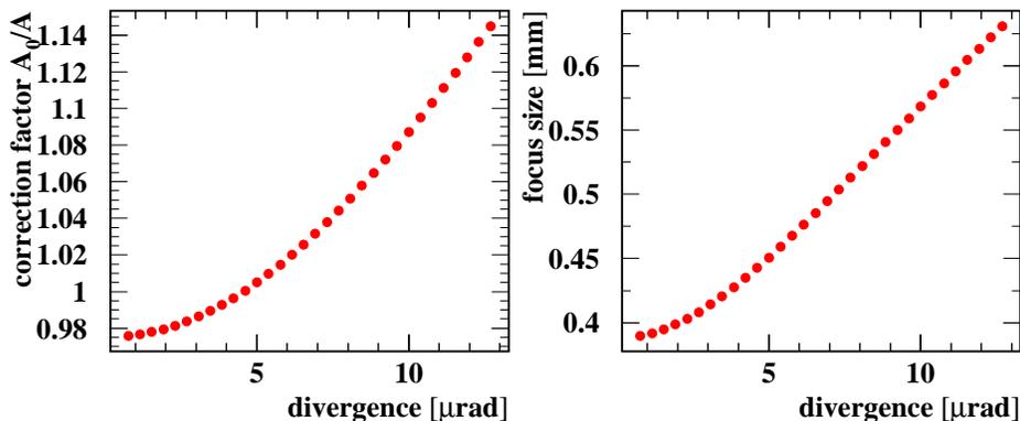
Figure 1: *Polarization correction factor and focus as a function of the angular divergence of the Compton beam for the HERA II detector setup. The Monte Carlo is tuned such that it is able to describe the risetime data if the HERA I detector configuration is selected.*
