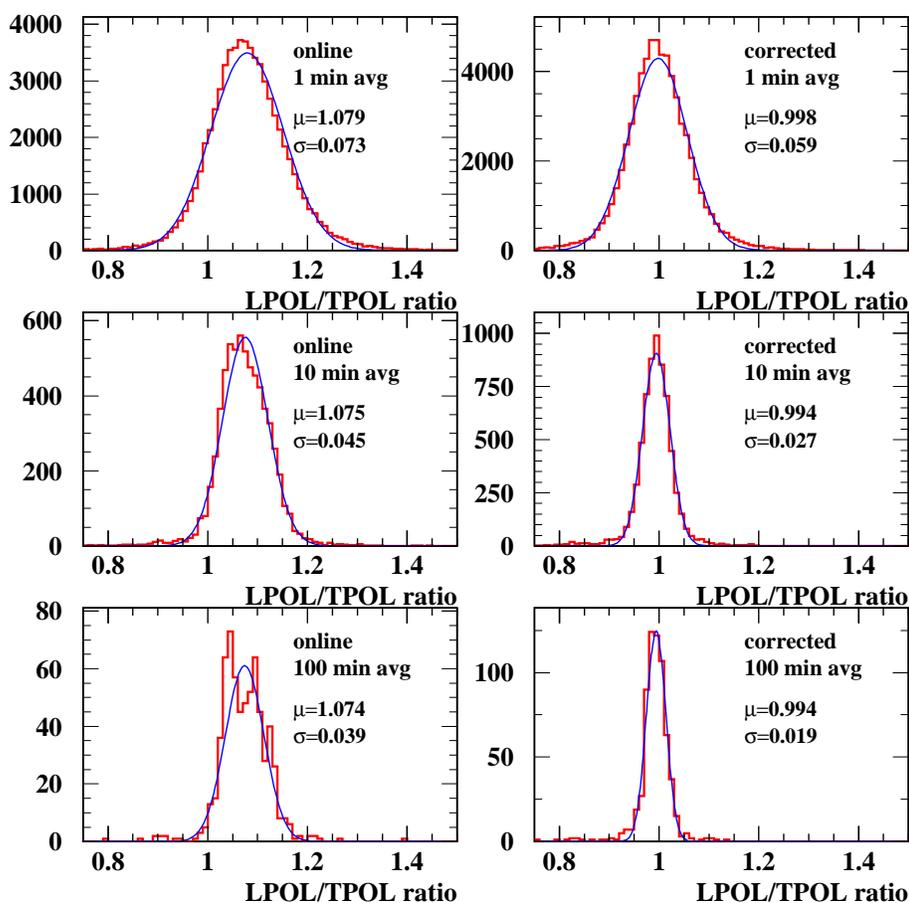
Figure 2: The ratio  $\frac{P_{LPOL}}{P_{TPOL}}$  for different averaging periods, shown on the left (right) without (with) the TPOL online measurement correction applied. Top: The average of 1 measurement (which takes 1 minute). Middle: The average of 10 consecutive measurements. Bottom: The average of 100 consecutive measurements.
