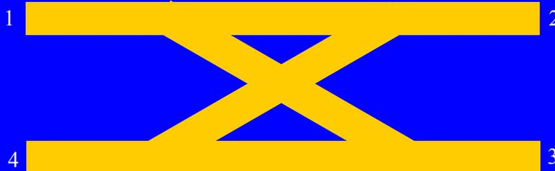
.Power from port 1 will be split and flow equally to ports 2 and 3, but with a phase shift.
