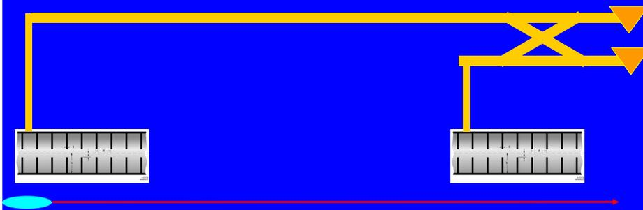
Beam and RF are synchronized at structure 1 if they both arrive at  $t=t_{\text{delay}}$
