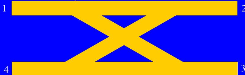
The key feature of the coupler is that the diagonal pathways are longer by  $90^\circ$  than the straight pathways. What does that do for us?
