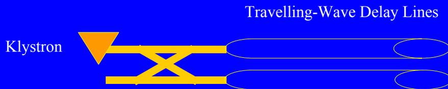
Same basic idea as SLED, but TE cavities are now very long compared to 1 wavelength -- can be treated as travelling-wave devices
