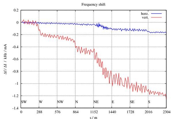
Figure 2: Measured intensity dependent frequency (beta-tron phase) shift along the PETRA III ring.
