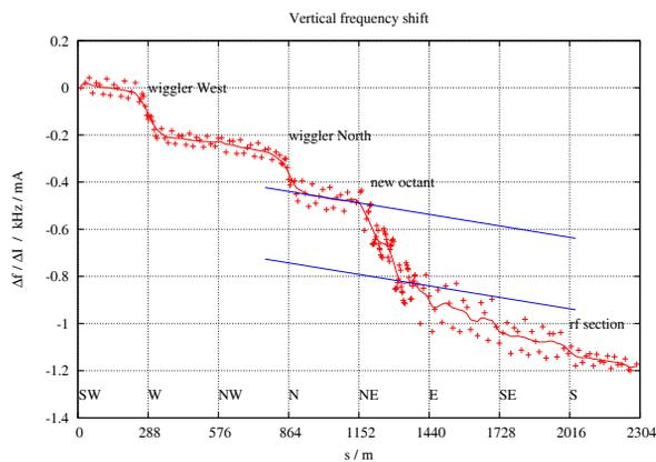
Figure 3: Measured intensity dependent vertical frequency (betatron phase) shift along the PETRA III ring. The crosses indicate the measured data at the beam position monitors. The solid line is a smoothed function through all the data points.
