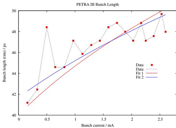
Figure 1: PETRA III bunch length (rms) versus bunch current. The measured data and two fits through the data points are shown.
