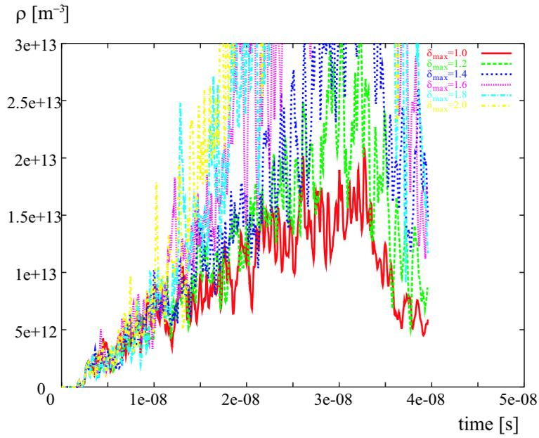
Figure 21: Central electron cloud volume density in units of  $\text{m}^{-3}$  as a function of time in s for a 1st order harmonic expansion of the CLIC wiggler field in Cartesian coordinates, assuming  $dN_{e^-}/dz = 0.11$  photoelectrons per  $e^+$  and meter; the various curves refer to six different values of  $\delta_{\text{max}}$ . Shown is the passage of 50 bunches followed by a gap.
