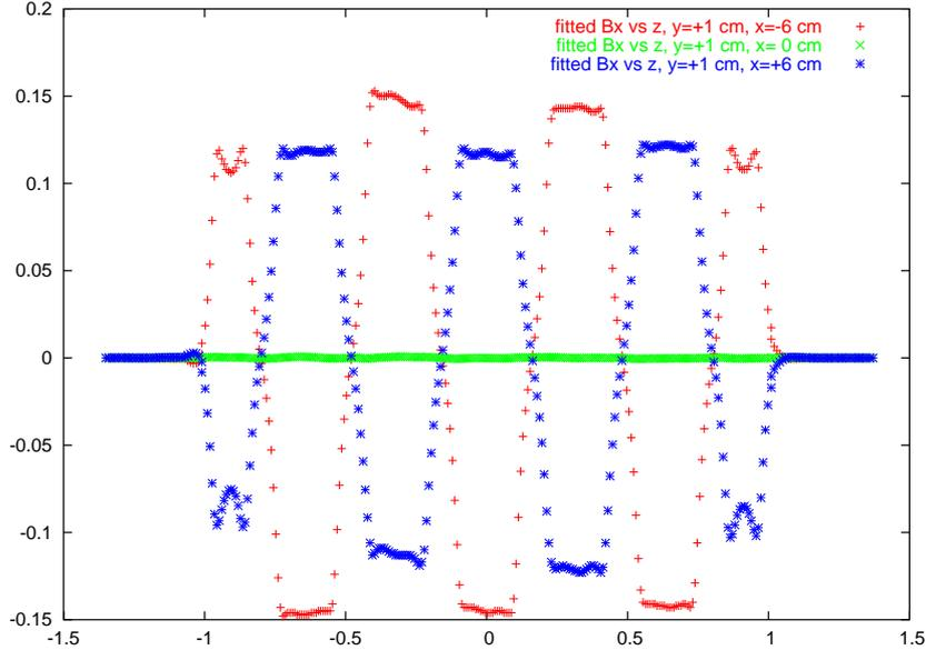
Figure 27: Horizontal magnetic field in the DAFNE wiggler after pole modification, reconstructed from a bi-cubic spline fit in the ECLLOUD code, as a function of longitudinal position. The top green curve refers to the horizontal center of the magnet, the red and blue curves show values measured with a horizontal offset of  $-6$  cm and  $+6$  cm, respectively, and a vertical offset of  $1$  cm.
