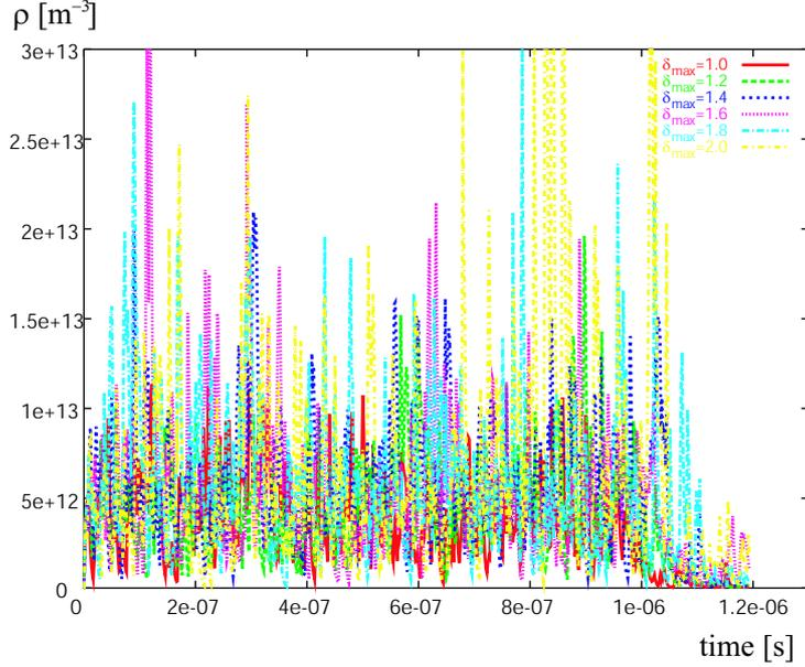
Figure 13: Central electron-cloud volume density in units of  $\text{m}^{-3}$  as a function of time in s for a 1st order expansion of the TESLA/ILC wiggler field in cylindrical coordinates, assuming  $dN_{e^-}/dz = 0.2$  photoelectrons per  $e^+$  and meter; the various curves refer to six different values of  $\delta_{\text{max}}$  [1].
