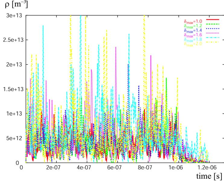
Figure 11: Central electron cloud volume density in units of  $\text{m}^{-3}$  as a function of time in s for a bending field whose strength is equal to the peak field of the TESLA wiggler, assuming  $dN_{e^-}/dz = 0.2$  photoelectrons per  $e^+$  and meter; the various curves refer to six different values of  $\delta_{\max}$ .
