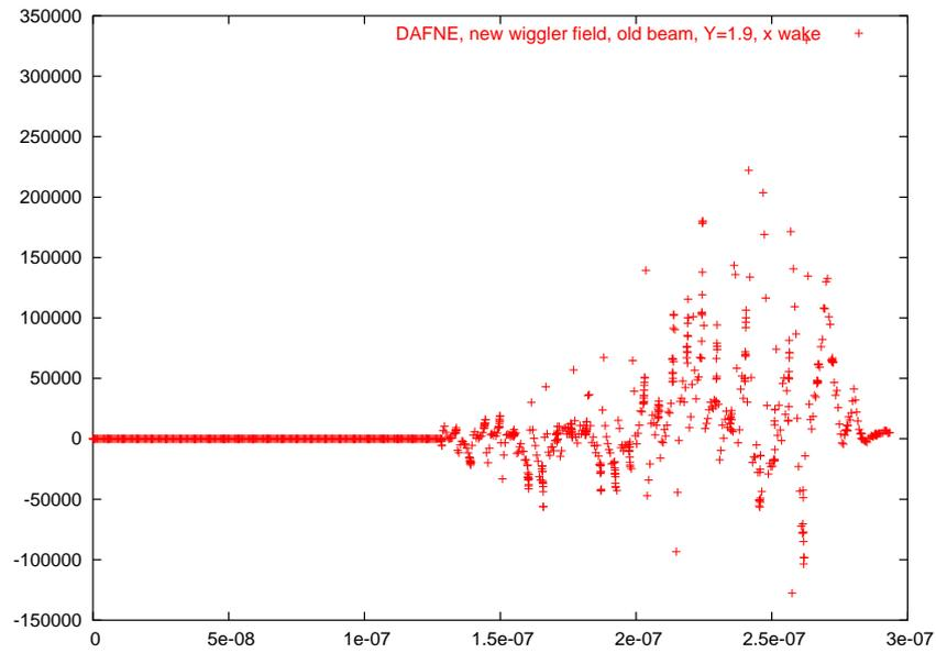
Figure 37: Multibunch wake field computed for the 2004 wiggler field and 2002 beam parameters. The 25th bunch of the train is displaced horizontally; the resulting wake field  $W$  for consecutive bunches is shown.
