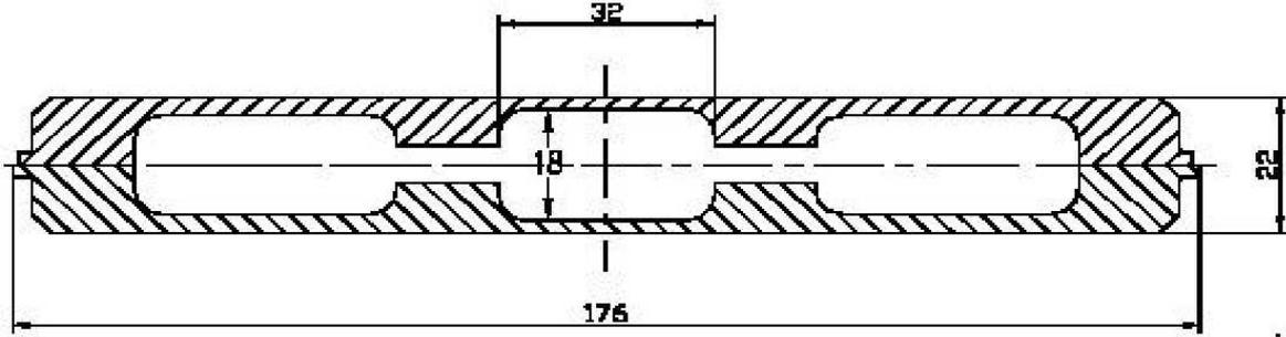
Figure 1: Model for vacuum chamber in TESLA/ILC or CLIC wiggler. The full height of the antechamber slot is taken to be 6 mm.
