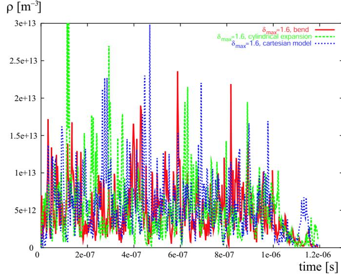
Figure 17: Central electron cloud volume density in units of  $\text{m}^{-3}$  as a function of time in s for  $\delta_{\text{max}} = 1.6$ , comparing the three different models of the TESLA/ILC wiggler field (constant bend, first term in a cylindrical expansion, first term in a harmonic expansion), assuming  $dN_{e^-}/dz = 0.2$  photoelectrons per  $e^+$  and meter.
