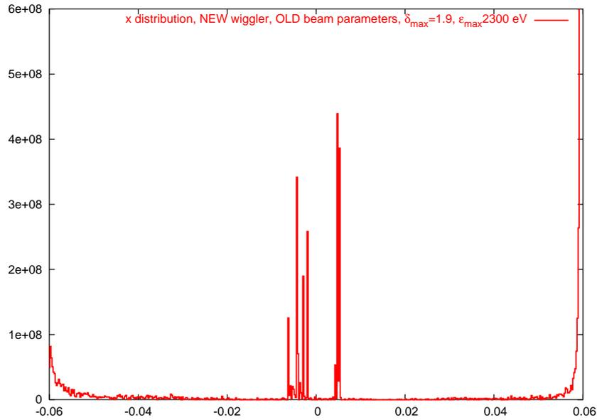
Figure 34: Horizontal electron distributions at the end of the simulation for the 2004/05 DAFNE wiggler with the 2002 beam parameters; we assumed a maximum secondary emission yield  $\delta_{\text{max}} = 1.9$  at  $\epsilon_{\text{max}} = 300$  eV, and  $dN_{e^-}/dz = 0.018$  photoelectrons per  $e^+$  and meter (twice the value of Table 1).
