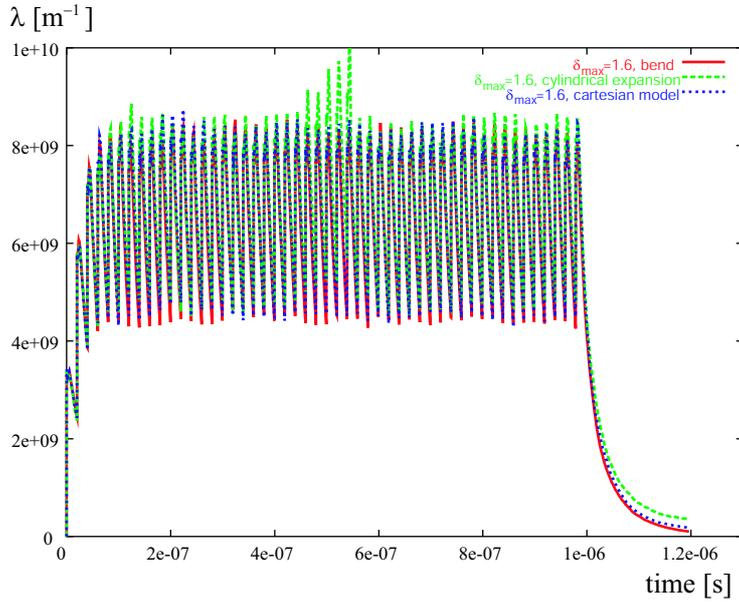
Figure 16: Electron line density in units of  $\text{m}^{-1}$  as a function of time in s for  $\delta_{\text{max}} = 1.6$ , comparing the three different models of the TESLA/ILC wiggler field (constant bend, first term in a cylindrical expansion, first term in a harmonic expansion), assuming  $dN_{e^-}/dz = 0.2$  photoelectrons per  $e^+$  and meter.
