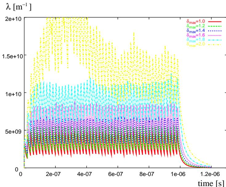
Figure 10: Electron line density in units of m<sup>-1</sup> as a function of time in s for a bending field whose strength is equal to the peak field of the TESLA/ILC wiggler, assuming  $dN_{e^-}/dz = 0.2$  photoelectrons per e<sup>+</sup> and meter; the various curves refer to six different values of  $\delta_{\max}$ .
