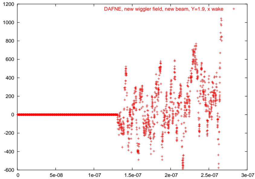
Figure 35: Multibunch wake field computed for the 2004 wiggler field and 2004 beam parameters. The 50th bunch of the train is displaced horizontally; the resulting wake field  $W$  for consecutive bunches is shown.
