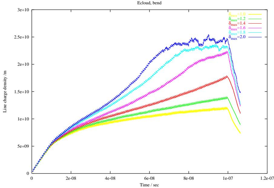
Figure 18: Electron line density in units of  $\text{m}^{-1}$  as a function of time in s for a bend with a field strength equivalent to the peak magnetic field strength of the CLIC wiggler magnet (1.76 T), assuming  $dN_{e^-}/dz = 0.11$  photoelectrons per  $e^+$  and meter; the various curves refer to six different values of  $\delta_{\text{max}}$ . Shown is the passage of 154 bunches followed by a gap.
