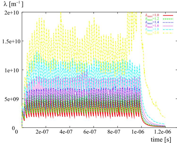
Figure 12: Electron line density in units of  $\text{m}^{-1}$  as a function of time in s for a 1st order expansion of the TESLA/ILC wiggler field in cylindrical coordinates, assuming  $dN_{e^-}/dz = 0.2$  photoelectrons per  $e^+$  and meter; the various curves refer to six different values of  $\delta_{\text{max}}$  [1].
