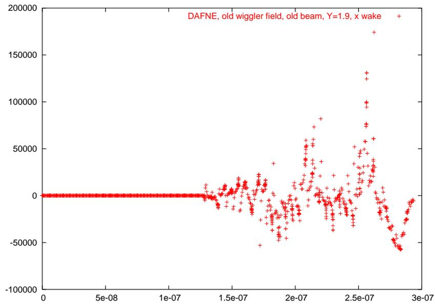
Figure 36: Multibunch wake field computed for the 2002 wiggler field and beam parameters. The 25th bunch of the train is displaced horizontally; the resulting wake field  $W$  for consecutive bunches is shown.
