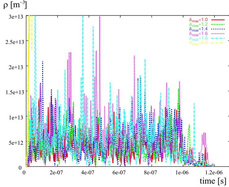
Figure 15: Central electron cloud volume density in units of  $\text{m}^{-3}$  as a function of time in s in a 1st order harmonic expansion of the TESLA/ILC wiggler field in Cartesian coordinates, assuming  $dN_{e^-}/dz = 0.2$  photoelectrons per  $e^+$  and meter; the various curves refer to six different values of  $\delta_{\text{max}}$ .
