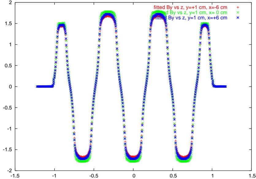
Figure 29: Vertical magnetic field in the DAFNE wiggler prior to pole modification, reconstructed from a bi-cubic spline fit in the ECLLOUD code, as a function of longitudinal position. The top green curve refers to the horizontal center of the magnet, the red and blue curves show values measured with a horizontal offset of  $-6$  cm and  $+6$  cm, respectively, and a vertical offset of  $1$  cm.
