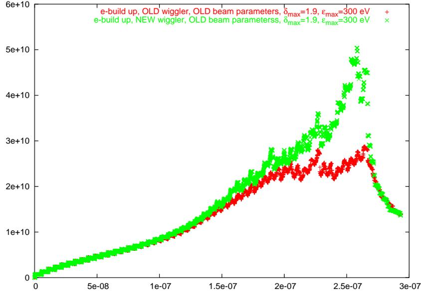
Figure 33: Simulated electron line density in units of  $\text{m}^{-1}$  as a function of time in s comparing the old and the new DAFNE wiggler, for the 2002 beam parameters; we assumed a maximum secondary emission yield  $\delta_{\text{max}} = 1.9$  at  $\epsilon_{\text{max}} = 300$  eV, and  $dN_{e^-}/dz = 0.018$  photoelectrons per  $e^+$  and meter (twice the value of Table 1).
