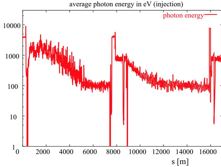
Figure 6: Average energy of photons (in eV) hitting the wall of the TESLA/ILC damping ring for beam parameters corresponding to injection (top) and extraction (bottom) [1], computed by PHOTON [3] (not counting photons absorbed in the antechamber).
