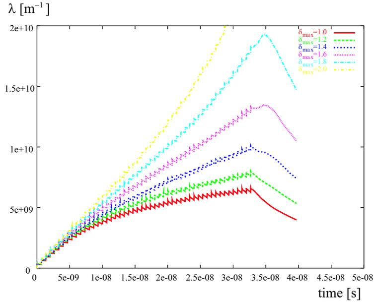
Figure 20: Electron line density in units of  $\text{m}^{-1}$  as a function of time in s for a 1st order harmonic expansion of the CLIC wiggler field in Cartesian coordinates, assuming  $dN_{e^-}/dz = 0.11$  photoelectrons per  $e^+$  and meter; the various curves refer to six different values of  $\delta_{\text{max}}$ . Shown is the passage of 50 bunches followed by a gap.
