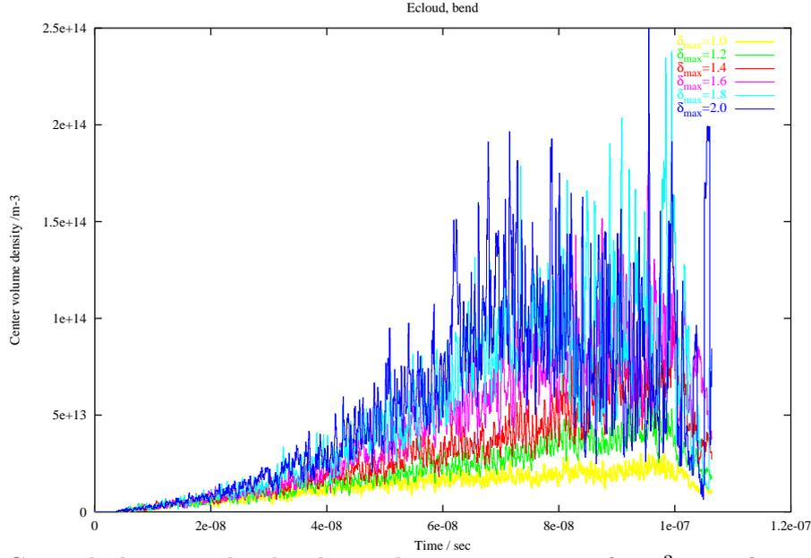
Figure 19: Central electron cloud volume density in units of  $\text{m}^{-3}$  as a function of time in s for a bend with a field strength equivalent to the peak magnetic field strength of the CLIC wiggler magnet (1.76 T), assuming  $dN_{e^-}/dz = 0.11$  photoelectrons per  $e^+$  and meter; the various curves refer to six different values of  $\delta_{\text{max}}$ . Shown is the passage of 154 bunches followed by a gap.
