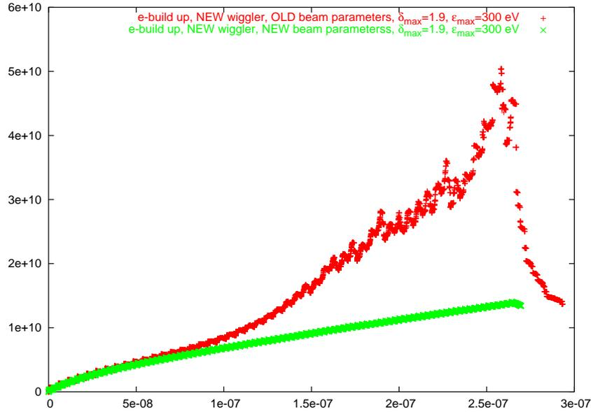
Figure 32: Simulated electron line density in units of  $\text{m}^{-1}$  as a function of time in s for the 2004 DAFNE wiggler with old and new beam parameters, assuming  $dN_{e^-}/dz = 0.018$  photoelectrons per  $e^+$  and meter (twice the value of Table 1),  $\delta_{\text{max}} = 1.9$  and  $\epsilon_{\text{max}} = 300$  eV.
