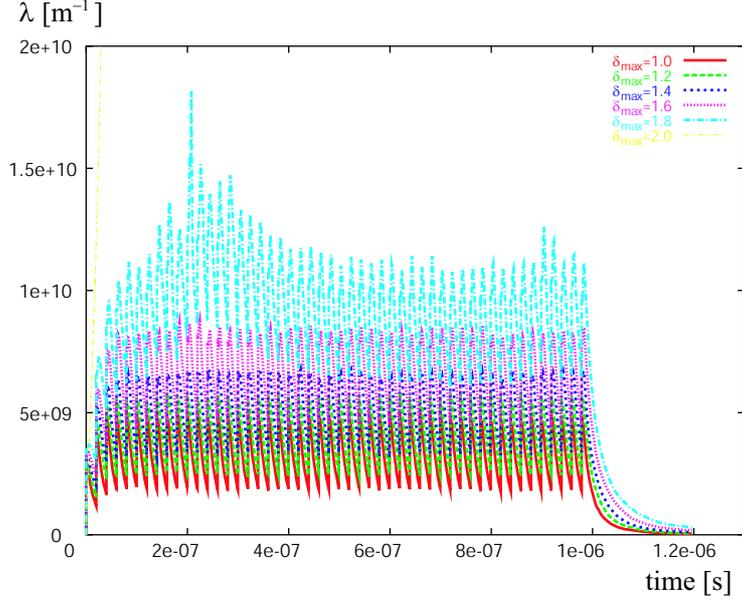
Figure 14: Electron line density in units of  $\text{m}^{-1}$  as a function of time in s in a 1st order harmonic expansion of the TESLA/ILC wiggler field in Cartesian coordinates, assuming  $dN_{e^-}/dz = 0.2$  photoelectrons per  $e^+$  and meter; the various curves refer to six different values of  $\delta_{\text{max}}$ .
