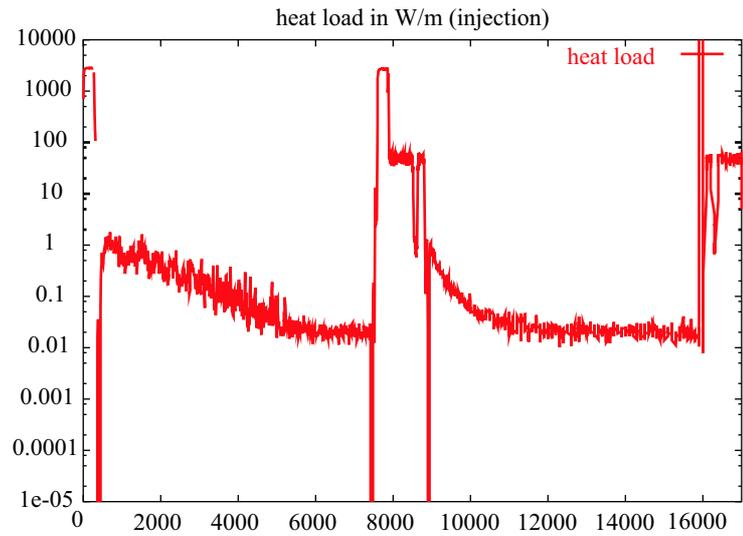
Figure 8: Synchrotron-radiation heat load on the wall of the TESLA/ILC damping ring for beam parameters corresponding to injection [1], computed by PHOTON [3] (photons absorbed in the antechamber were not counted).
