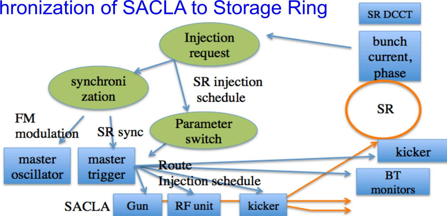
Prototype of the synchronization system tested at SACLA.
