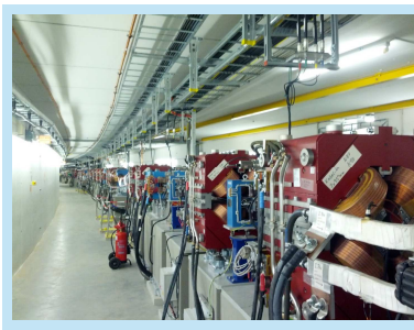
Figure 5: The new DBA like lattice of the extension section North is shown in the photo from April 2015.
