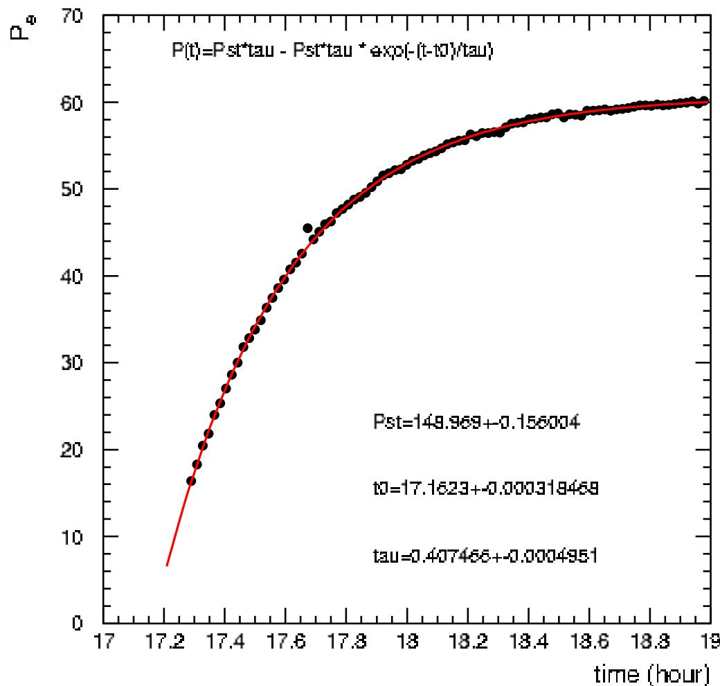
3 pairs of rotators (so max. Sokolov-Ternov polarisation = 83 %), solenoids on, no beam-beam
